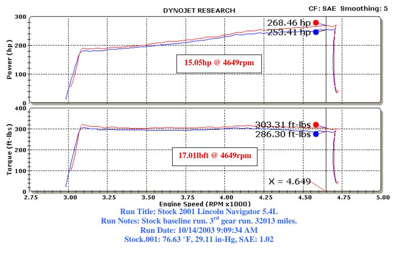
Run Title: K&N 2001 Lincoln Navigator 5.4L Run Notes: K&N intake kit #57-2558 installed. 3<sup>rd</sup> gear run. 32013 miles. Run Date: 10/14/2003 10:43:18 AM K&N.002: 82.11 °F, 29.06 in-Hg, SAE: 1.03
