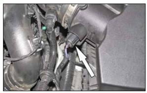
2. Disconnect the Inlet air temperature sensor electrical connection.
