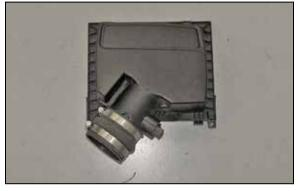
16. Install the remaining hump hose (087121) onto the factory air box as shown and secure with the provided hose clamp.
