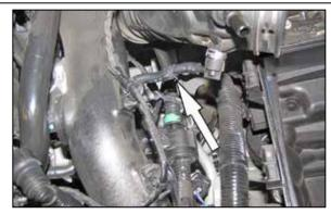
6. Disconnect the solenoid vent hose from the fitting installed into the factory intake tube.
