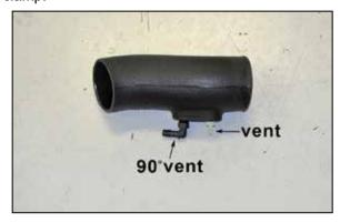
9. Install the provided 1/4npt vent fittings into the K&N® intake tube as show.
