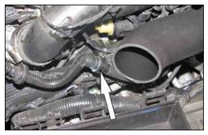
14. Connect the factory crank case vent hose to the guick connect fitting/vent hose installed into the K&N® intake tube.
