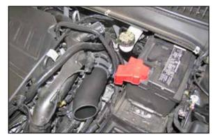
13. Install the K&N® intake tube into the coupling hose at the turbo but do not tighten at this time.
