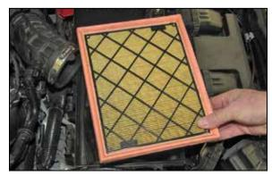
5. Release the two upper air box retaining clips and then remove the upper air box and stock air filter.
