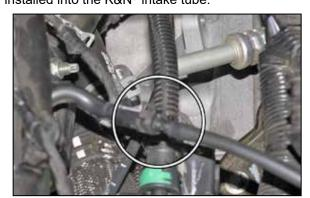
12. Set the intake tube in and then connect the solenoid vent hose to the hose installed onto the K&N® intake tube
