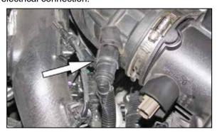
3. Disconnect the crank case vent connection.
