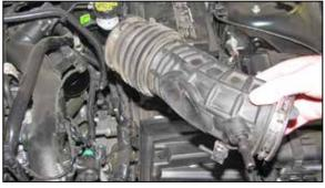
7. Loosen the hose clamp securing the factory intake tube to the turbo inlet and then remove the hose from the vehicle.
