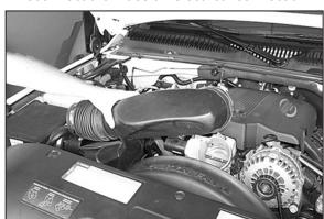
3. Loosen the hose clamps at the throttle body and at the mass air sensor, then remove the factory intake tube as shown.
