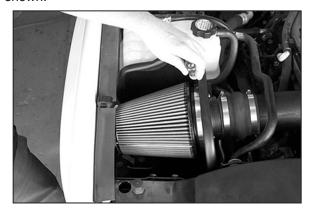
13. Install the K&N® Air Filter onto the mass air adapter, then tighten the hose clamp as shown. NOTE: Drycharger® air filter wrap; part # RF-1041DK is available to purchase separately. To learn more about Drycharger® filter wraps or look up color availability please visit http://www.knfilters.com®.
