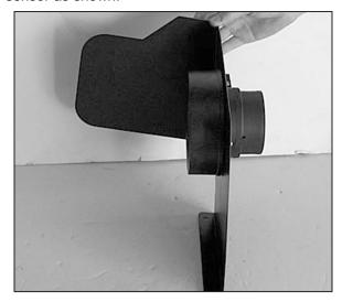
6. Using the provided hardware, assemble the the mass air sensor, gaskets, heat shield and mass air sensor as shown.
