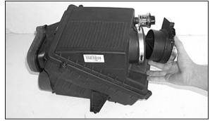
5. Loosen the hose clamp and remove the mass air sensor as shown.
