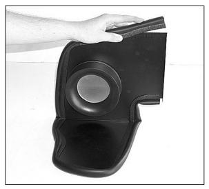
7. Apply the provided trim seal to the heat shield assembly as shown.
