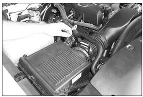
2. Disconnect the mass air electrical connection.
