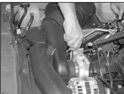
4. Loosen the hose clamp at the throttle body.
