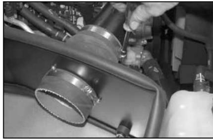
21. Install the intake tube onto the vehicle; then align the tube with the mass air sensor and then tighten hose clamp.
