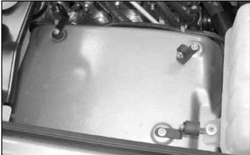
15. Install the 3 brackets onto the vehicle with the provided hardware as shown. Don't tighten completely at this time.
