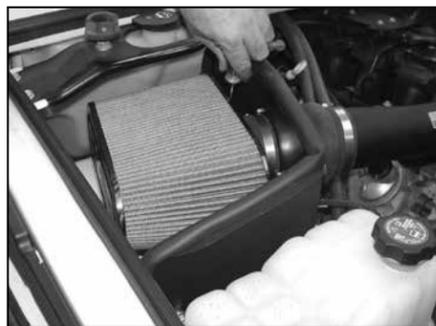
23. Install the air filter onto the mass air sensor and then tighten hose clamp.
