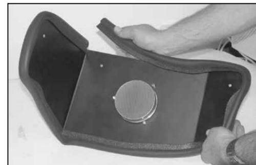
11. Install the edge trim onto the heat shield. **NOTE: Some trimming of the edge trim may be necessary.**
