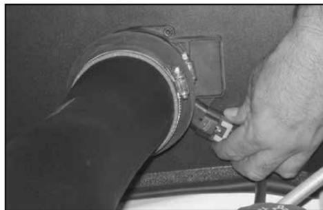
24. Reconnect the mass air electrical connection as shown.
