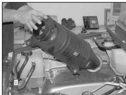
8. Remove the air box from vehicle as shown. **NOTE: K&N Engineering, Inc., recommends that customers do not discard factory air intake.**
