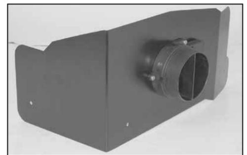
10. Install the mass air sensor onto the heat shield with the provided hardware.
