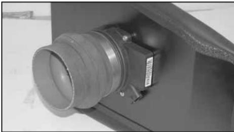
16. Install the silicone hump hose (08176) onto the mass air sensor with the provided hose clamps as shown.
