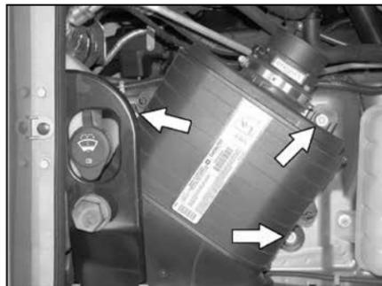
7. Remove the 3 10mm bolts that retain the air box onto the vehicle.
