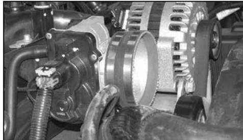
20. Install the provided silicone hose (08755) onto the throttle body with provided hose clamps.
