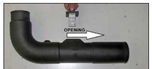
16. Install the mass air sensor assembly into the K&N® intake tube and secure with the provided hardware.
