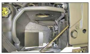
9. Install the heat shield and secure it to the air filter housing mounting plate location using three of the factory bolts from step #7.
