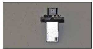
15. Remove the two screws securing the mass air sensor into the air filter housing and then remove the mass air sensor from the air filter housing. Install the mass air sensor into the K&N® adapter and secure with the provided hardware.
