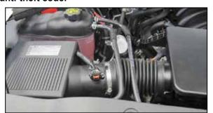
2. Disconnect the mass air sensor electrical connection and unhook the wiring harness from the air filter housing.
