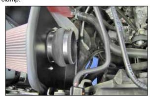
13. Install the provided hump hose (08418) onto the filter adapter and secure with the provided hose clamp.
