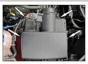
5. Loosen the four screws that secure the upper air filter housing and then remove the upper housing and set aside.
