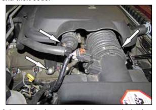
2. Loosen the hose clamp that secures the intake hose to the air filter housing. Using a screwdriver, unlock the small clamp the secures the vent line to the connector and then disconnect the vent line. Remove the bolt securing the intake plenum to the engine.
