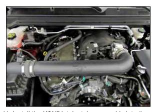
11. Install the K&N® intake tube assembly into the coupler on the air filter housing and then into the coupler at the throttle body, adjust the tube for best fit and then secure with the provided hose clamps.
