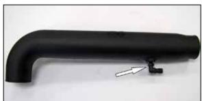
10. Install the provided 90° vent fitting into the K&N® intake tube as shown.
