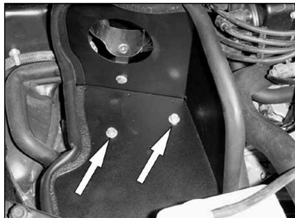
16. Attach the heat shield to the rubber mounted studs on the "Z" bracket using the hardware provided.
