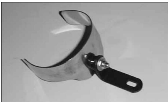
10. Assemble the saddle and "L" bracket using the hardware provided.
