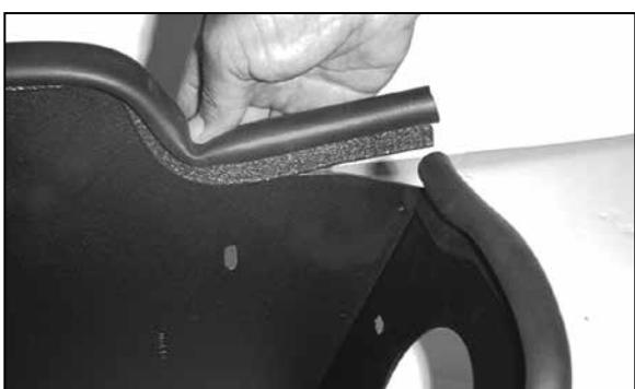
11. Install the trim seal onto the heat shield as shown.
