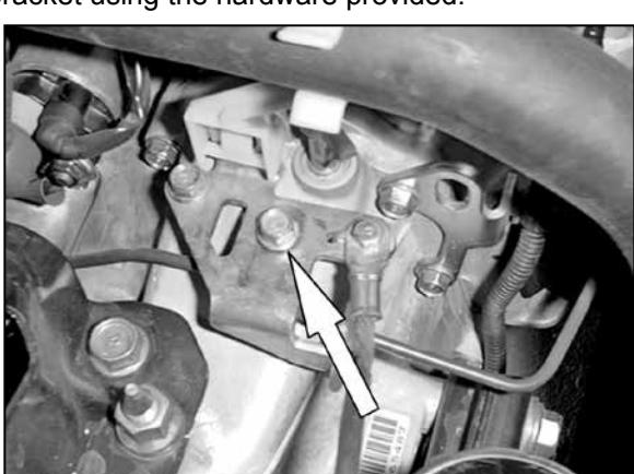
14. Loosen and remove the bolt that retains the transmission hanger to the transmission.
