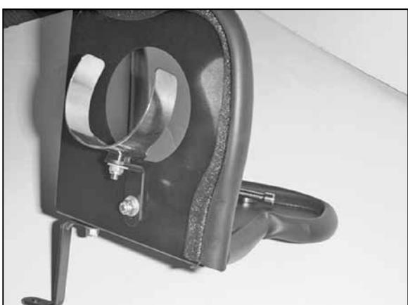
12. Attach the saddle bracket assembly to the heat shield using the hardware provided.
