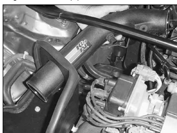
18. Install the K&N® intake tube, feeding the straight end through the hole in the heat shield.
