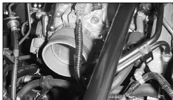
17. Attach the silicone hose to the throttle body using the hose clamp provided.
