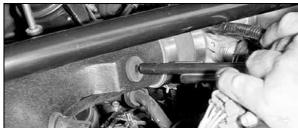
21. Insert the crankcase vent hardline into the grommet in the K&N® intake tube.
