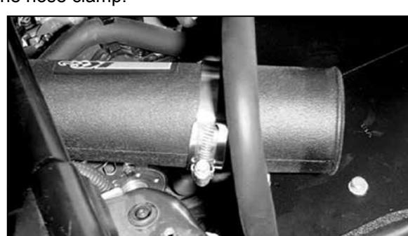
20. Secure the saddle bracket to the intake tube using the hose clamp provided.
