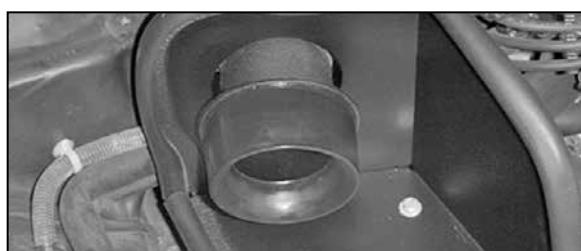
22. Install the adapter onto the K&N® intake tube.
