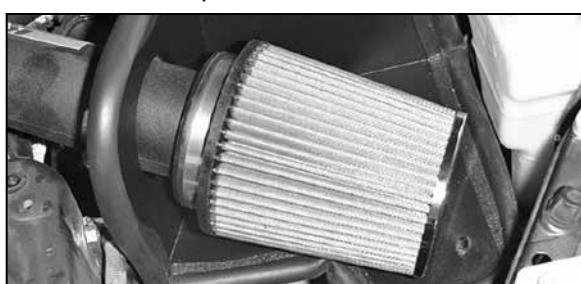
23. Install the Filtercharger element and tighten hose clamp.
