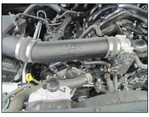
10. Install the K&N® intake tube into the hump coupler at the air filter housing lid and then into the coupler at the throttle body, resecure the air filter housing lid, adjust the tube for best fit and then secure the hose clamps.
