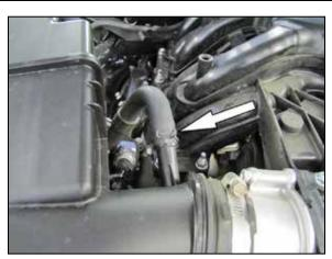
3. Release the spring clamp and disconnect the crank case vent hose from the factory intake tube.
