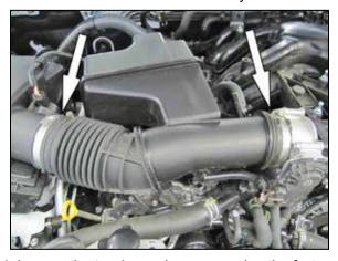
4. Loosen the two hose clamps securing the factory intake tube and then remove the intake tube from
