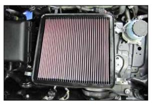
5. Release the clips securing the upper air filter housing to the lower air filter housing. Lift up the upper air filter housing and remove it from the vehicle. Remove the factory air filter. Install the K&N® air filter into the lower air filter housing and then reinstall the upper air filter housing but do not secure at this time.
