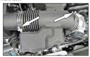
4. Loosen the hose clamps securing the factory intake tube to the throttle body and air filter housing and then remove the factory intake tube from the
