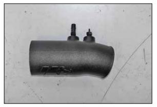
8. Install the provided NPT vent fittings into the K&N® intake tube as shown.
