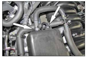
3. Disconnect the crank case vent hose and fuel pressure regulator vent hose from the factory intake tube.
