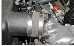
6. Install the provided coupling hose (08760) onto the air filter housing and secure with the provided hose clamp.
