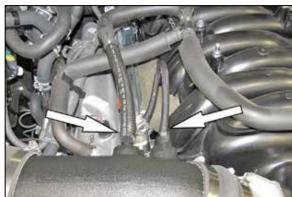
11. Connect the union into the factory crank case vent hose and then connect the open end onto the fitting installed into the K&N® intake tube. Then connect the fuel pressure regulator vent hose to the fitting installed in the K&N® intake tube.
