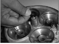
Apply spacer onto carburetor center post.
