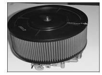
13) Once installation is completed, make sure that the arrow on the top plate is still facing in the proper direction.
