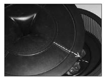
Place the Flow Control top onto the Filtercharger with the arrow pointing forwards or backwards to the float bowl vents.
