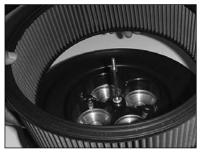
7) Place the K&N Fllterc,harger onto the base plate.
