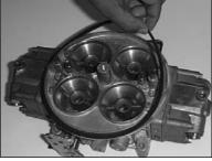
Apply the provided K&N gasket onto carburetor.
