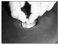
12) Place the provided nylock nut onto the stud and tighten down completely.
