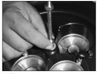
Place stud onto center post and tighten snug. NOTE: to avoid damage to the K&N Flow Control Stub Stack, do not over tighten.
