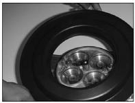
3) Place K&N base plate onto carburetor.
