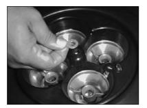
5) Place the small flat metal washer onto the K&N Stub Stack.
