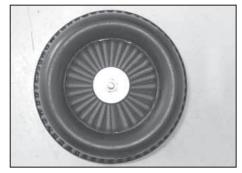
28. Install the provided bolt through the air filter top
