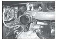
21. Install the K&N<sup>®</sup> intake tube into the factory rubber manifold and secure with the factory clamp removed in step #18 as shown.
