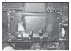
39. Re-install the engine splash cover as shown.
