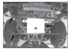
12. Remove the heat shield and both cargo bed brackets shown.
