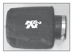
30. Install the K&N<sup>®</sup> Drycharger<sup>®</sup> onto the K&N<sup>®</sup> air filter (with the bolt protruding through the reinforcement patch) as shown.
