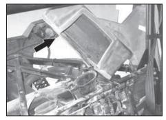
14. Remove the intake cover as shown.
