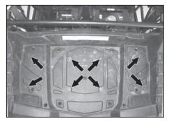
7. In the cargo bed, remove the four 13mm bolts and four torx bolts as shown.
