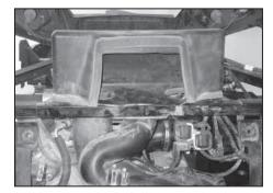
33. Re-install the plastic intake cover using the factory clips (removed in step #12).
