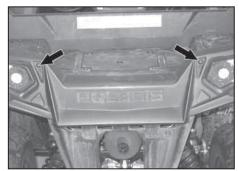
38. Re-install the two bolts securing the rear of the cargo bed as shown.
