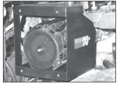
31. Install the K&N<sup>®</sup> air filter assembly and secure it with the provided hose clamp.
