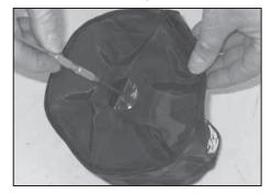
29. Using a sharp tool, poke a hole in the center of the reinforcement patch on the K&N<sup>®</sup> Drycharger<sup>®</sup>.
