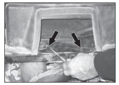
13. Remove the two push pins that secure the intake cover as shown.
