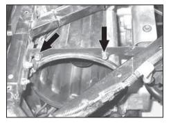
17. Remove the two 13mm bolts that secure the upper air box assembly to the upper air box mount as shown.
