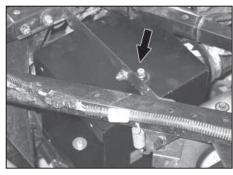
25. Install the K&N<sup>®</sup> air box assembly, aligning it with the lower air box mounting bracket and K&N<sup>®</sup> intake tube. Align the upper air box bracket with the stock air box mount and secure it with the provided hardware as shown. Then, secure the air box to the lower mounting bracket (installed in step #20).
