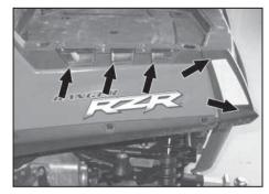
10. Remove the five screws located inside the fender (that secure the left side fender onto the cargo bed) as shown.
