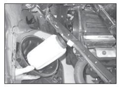
15. Loosen the two air filter cover snaps. Remove the air filter cover and air filter as shown.
