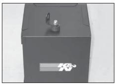
23. Install the bracket assembly (from step #22) onto the K&N $^{\circ}$  air box with the provided hardware as shown.
