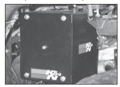
32. Install the K&N<sup>®</sup> air box cover, aligning the  $\frac{1}{4}$ " bolt in the filter with the center hole in the cover on the K&N<sup>®</sup> air box. Secure with the provided hardware as shown.
