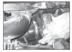
18. Loosen the hose clamp at the rear of the air box (at the factory rubber manifold) as shown. **NOTE: The clamp will be re-used in step #21.**
