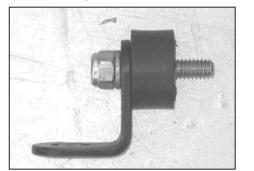
22. Install the provided rubber mounted stud onto the upper air box bracket (#070066) as shown.
