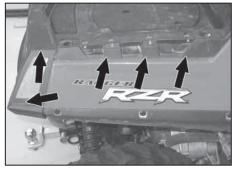
36. Re-install the five screws securing the right side fender onto the cargo bed as shown.
