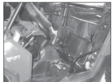
2. Remove the driver and passenger seats as shown.
