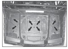
35. Align the cargo bed with the factory heat shield and cargo bed brackets. Secure the cargo bed with the four 13mm and the four torx bolts as shown.
