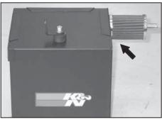
24. Install the K&N<sup>®</sup> crank case vent filter onto the air box assembly with the provided hardware as shown.
