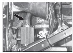
26. Install the crank case vent tube into the K&N $^{\otimes}$  crank case filter as shown.
