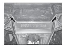
8. Remove the two torx bolts at the rear of the cargo bed as shown.
