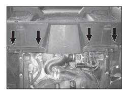
5. Remove the four bolts securing the front of the cargo bed as shown.
