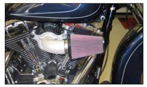
13. Install the K&N® air filter onto the intake tube and secure with the provided hose clamp. A black hose clamp is being supplied with kit. This clamp is intended to clamp the filter to the intake tube.
