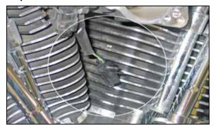
7. Using the provided tie wrap, secure the loose pig tail to the to the throttle position switch wiring harness.
