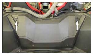
2. Unlock the two quarter turn fasteners and then remove the air filter access panel.
