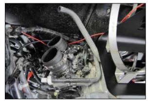
13. Install the two provided couplers onto the throttle bodies as shown and secure with the provided hose clamps.
