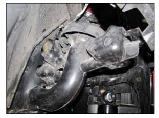
4. Loosen the hose clamp and retaining clips that secure the fresh air intake duct and then remove the duct.
