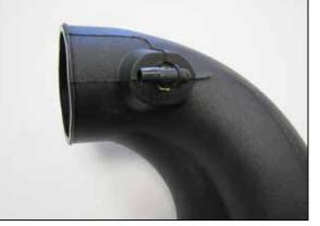
12. Install the 90deg vent fitting into the K&N intake tube as shown.
