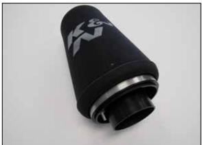
19. Install the K&N air filter onto the filter adapter and secure with the provided hose clamp, then install the foam filter wrap onto the air filter.
