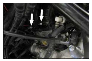
5. Loosen the two hose clamps that secure the intake hose to the throttle bodies.
