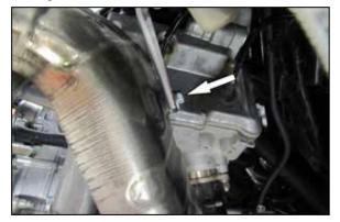
8. Remove the bolt that secures the air filter housing bracket to the exhaust.
