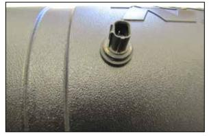
16. Remove the inlet air temperature sensor from the factory air filter housing and install it into the grommet installed into the K&N housing.
