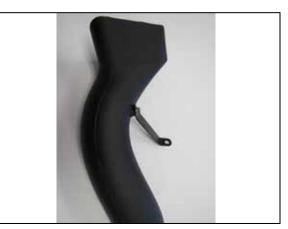
26. Install the fresh air duct mounting bracket onto the K&N fresh air duct using the provided hardware.
