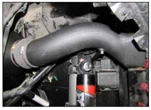
27. Install the fresh air duct into the coupler and then align the bracket, adjust the duct for best fit and then secure with the provided hardware and hose clamps.
