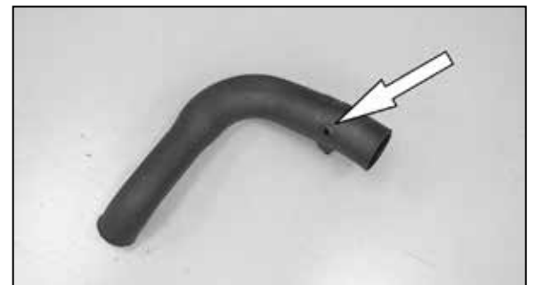
20. Install the provided grommet into the K&N® intake tube as shown.
