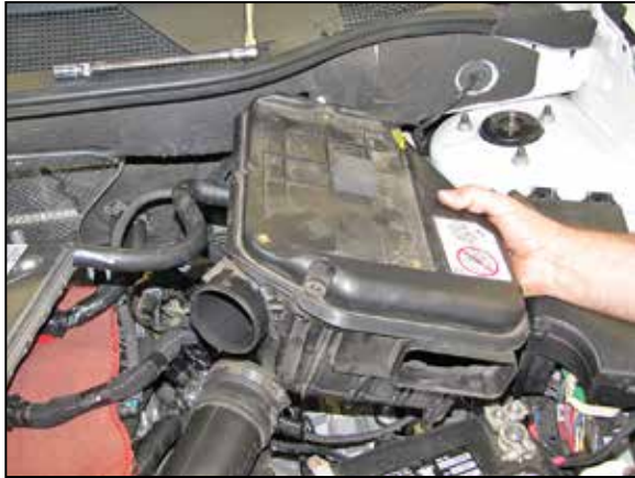
8. Lift up the air box to dislodge it from the mounting grommets and then remove it from the vehicle.
