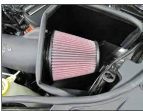
15. Install the K&N® air filter onto the intake tube and secure with the provided hose clamp. NOTE: Drycharger® air filter wrap; part # RF-1042DK is available to purchase separately. To learn more about Drycharger® filter wraps or look up color availability please visit http://www.knfilters.com®.
