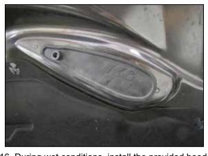
16. During wet conditions, install the provided hood vent block off to minimize water intrusion to the intake system.
