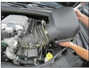
4. Lift the air filter housing assembly up to release it from the mounting grommets and then remove the complete intake system from the vehicle.
