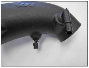
12. Remove the O-ring from the IAT sensor and then install the sensor into the K&N® intake tube as shown. Install the factory quick connect CCV fitting into the K&N® intake tube as shown.
