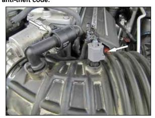
2. Disconnect the IAT sensor electrical connection. Disconnect the CCV hose from the quick connect fitting.
