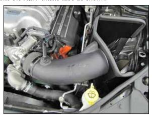
13. Install the K&N® intake tube into the heat shield and coupler as shown and secure with the hardware and hose clamp provided.
