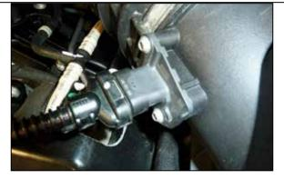
Release the locking tab and then disconnect the mass air sensor electrical connection.
