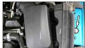
6. Remove the bolt that secures the factory air filter housing to the vehicle and then remove the housing from the vehicle.
