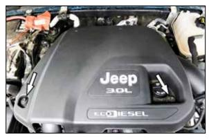
2. Remove the two bolts that secure the engine cover and then remove the engine cover from the vehicle.
