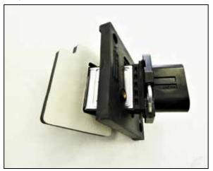
11. Install the mass air sensor adapter gasket onto the adapter. Remove the mass air sensor from the factory housing and then install it into the K&N adapter and secure with the provided hardware.
