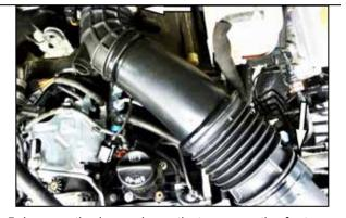
5. Loosen the hose clamp that secures the factory intake hose to the turbo inlet, then release the plastic clamp that secures the hose to the factory air filter housing. Remove the factory intake hose from the vehicle.
