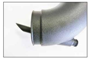
12. Install the provided CCV vent tube into the K&N intake tube as shown. NOTE: Be sure it is positioned as shown for proper function.
