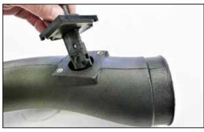
13. Install the mass air sensor assembly into the K&N intake tube and secure with the provided hardware. NOTE: be sure to install the sensor in the correct direction, see photo.
