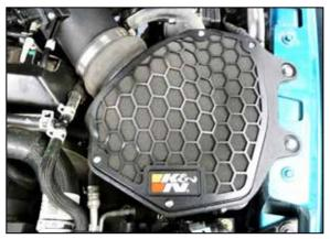
18. Assemble the foam filter and cage assembly and secure it to the air filter housing with the provided hardware.
