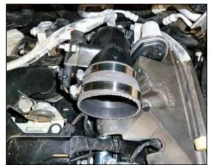
10. Install the provided straight coupler onto the turbo inlet and secure with the provided hose clamp.
