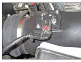
35. Reconnect the mass air sensor electrical connection. Secure the mass air sensor wiring harness to the A/C recharge pipe with the provided tie wrap.
