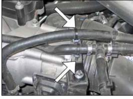
34. Secure the two coolant hoses with the provided mounting tie wraps as shown.
