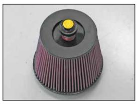
37. Install the filter minder along with the provided grommet into the K&N® air filter as shown.
