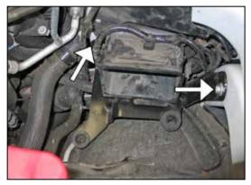
12. Remove the two bolts that secure the air box mounting bracket to the core support and inner fender.
