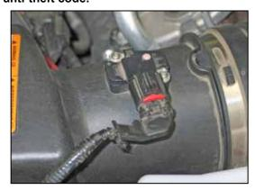
2. Release the red locking tab and then disconnect the mass air sensor electrical connection and unhook the wiring harness from the air box.
