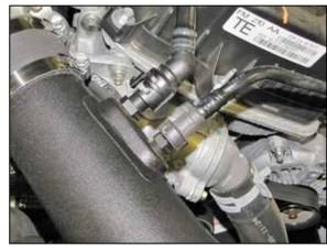
15. Connect the crank case vent and EVAP vent lines to the fittings installed into the K&N® intake tube
