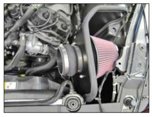
11. Install the provided hump coupler (08699) onto the filter adapter and secure with the provided hose
