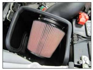
20. Install the K&N<sup>®</sup> air filter onto the intake tube and secure with the provided hose clamp. NOTE: Drycharger<sup>®</sup> air filter wrap; part # RC-5139DK is available to purchase separately. To learn more about Drycharger<sup>®</sup> filter wraps or look up color availability please visit
