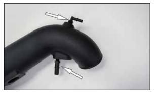
9. Install the provided fittings into the K&N<sup>®</sup> intake tube as shown.
