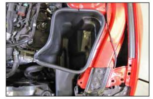
8. Install the provided edge trim onto the K&N® air filter housing. Install the K&N® air filter housing into the vehicle and secure with the provided hardware. NOTE: Some trimming of the edge trim will be necessary.
