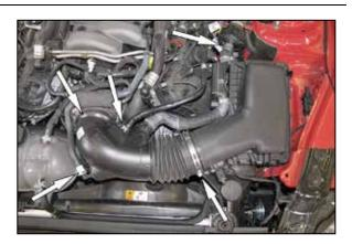
5. Disconnect the EVAP vent line, cut the clamp for the sound tube at the sound drum and disconnect the hose from the drum. Loosen the hose clamps that secure the intake tube to the throttle body and air filter housing then remove the intake tube from the vehicle.
