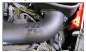
15. Install the intake tube into the coupler at the throttle body and onto the filter adapter, secure the tube to the filter adapter with the provided hardware and to the coupling hose with the provided hose clamp.
