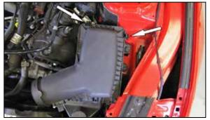
6. Release the clips that secure the upper air filter housing and then remove the upper air filter housing from the vehicle.
