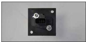
11. Remove the mass air sensor from the factory air filter housing and install it into the K&N® adapter using the provided hardware.
