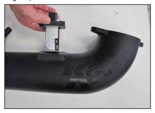
12. Install the mass air sensor assembly into the K&N® intake tube as shown and secure with the provided hardware.
