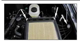
7. Disconnect the wiring harness and purge solenoid from the lower air filter housing if equipped. Remove the bolt that secures the lower air filter housing to the inner fender and then remove the lower housing from the vehicle.
