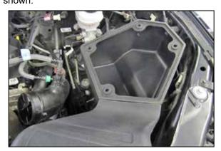
12. Install the K&N® lower air filter housing assembly into the vehicle so the mounting studs insert into the factory mounting grommets and it aligns with the rubber mounted stud installed into the inner fender. Secure the assembly with the hardware and clips provided.
