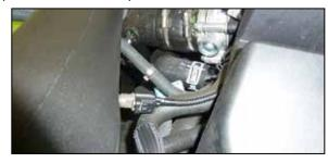
20. Reconnect the inlet air temperature sensor electrical connection using the provided extension
