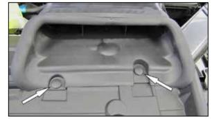
6. Release the two clips that secure the factory fresh air intake duct to the core support.
