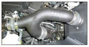
19. Install the K&N® intake tube into the couplers for the turbo inlet pipes and the filter adapter, adjust the tube for best fit and then secure with the provided hose clamps.
