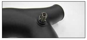
18. Remove the inlet air temperature sensor from the factory intake tube and remove the O-ring from the sensor. Using the provided grommet, install the inlet air temperature sensor into the K&N® intake tube as shown.
