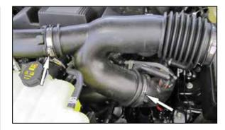
5. Loosen the two remaining hose clamps that secure the factory intake tube to the turbo inlet pipes and then remove the intake tube from the vehicle.
