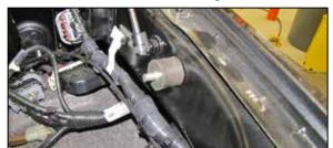
11. Install the rubber mounted stud into the factory inner fender air filter housing mounting location as
