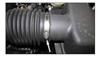
3. Loosen the hose clamp that secures the factory intake tube to the factory upper air filter housing.
