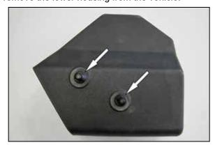
8. Install the two mounting studs provided into the K&N® lower air filter housing as shown using the provided hardware.
