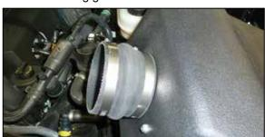
16. Install the provided hump coupler (08699) onto the filter adapter and secure with the provided hose clamp.
