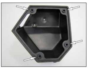
9. Install the four mounting grommets provided into the K&N® lower air filter housing as shown.
