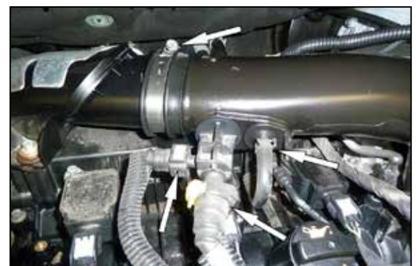
5. Disconnect the three EVAP and CCV vent lines from the intake tube, then loosen the hose clamp that secures the intake tube to the turbo inlet tube.
