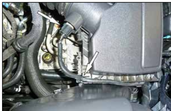
4. Disconnect the inlet air temperature electrical connection and then unhook the wiring harness from the air filter housing.
