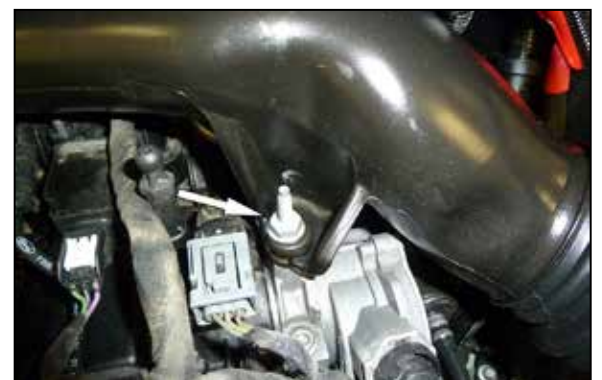
6. Remove the bolt that secures the intake tube to the engine.
