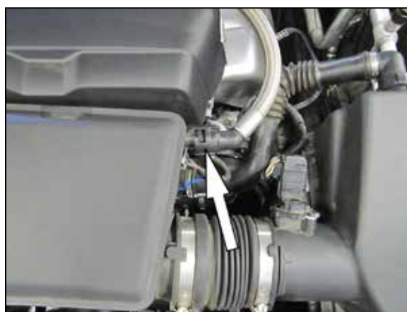
3. Disconnect the Crank case vent hose from the intake plenum.
