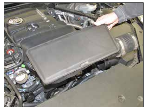
5. Remove the intake plenum from the vehicle.
