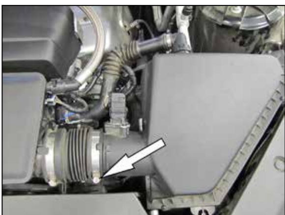
2. Loosen the hose clamp securing the intake tube to the air filter housing.
