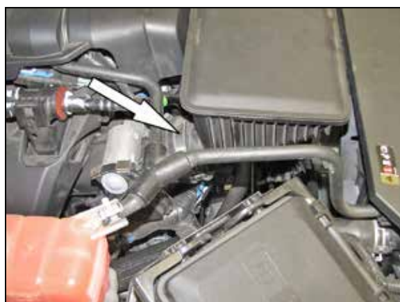
4. Loosen the hose clamp securing the intake plenum to the throttle body.
