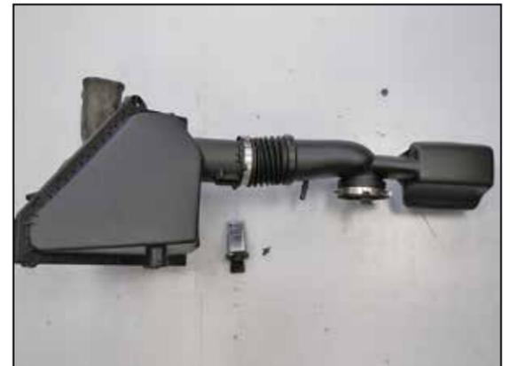
18. Remove the sensor from the factory intake system.
