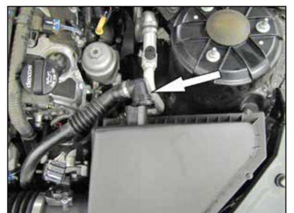
5. Release the air injection quick disconnect fitting and then disconnect the air injection tube from the factory air box.
