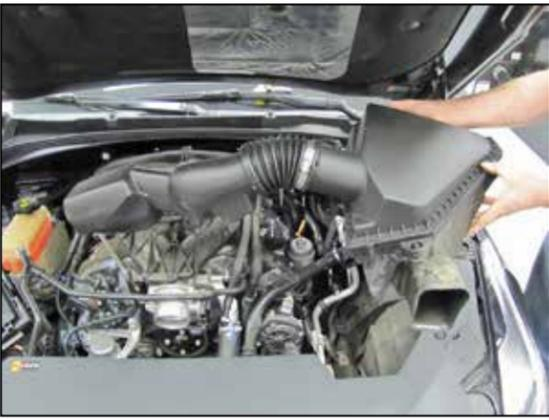
7. lift up the air filter housing to dislodge it from the mounting grommets and then remove the complete factory intake system.
