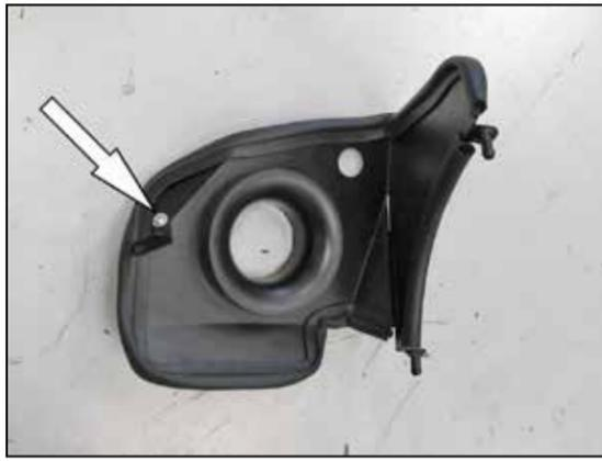
12. Install the provided heat shield mounting bracket (064319) onto the heat shield using the provided hardware.
