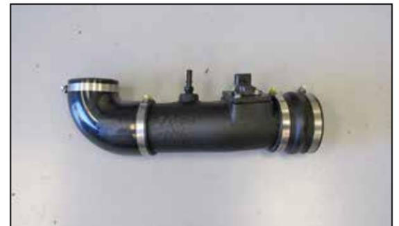
21. Install the provided angle hose #08629 and hump hose #08493 onto the K&N® intake tube but do not completely tighten at this time.
