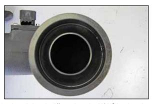
17. Install the air diffuser into the K&N® intake tube so the radiused surface is located inside the tube.
