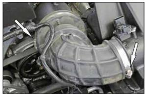
3. Loosen the two hose clamps that secure the intake tube to the turbo inlet and air filter housing. And then remove the intake tube from the vehicle.
