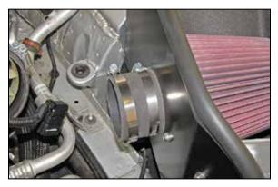
12. Install the provided coupler hose (08711) onto the filter adapter and secure with the provided hose
