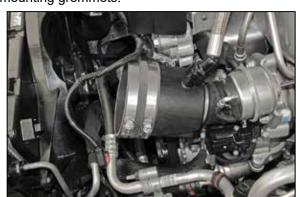
11. Install the provided coupler hose (08540) onto the turbo inlet chamber and secure with the provided hose clamp.
