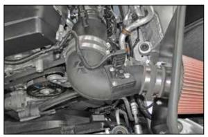
18. Install the Intake tube into the coupler at the filter adapter and then into the coupler at the turbo inlet chamber, adjust the tube and heat shield for best fit and then secure with the provided hose clamps. Reconnect the mass air sensor electrical connection and secure the wiring harness to the insert in the intake tube.
