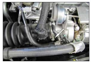
4. Loosen the hose clamp that secures the intake tube to the turbo inlet then disconnect the tube from the turbo. Lift the intake assembly up to dislodge it from the mounting grommets and then remove the complete intake system from the vehicle. NOTE: K&N Engineering, Inc., recommends that customers do not discard factory air intake.
