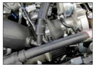
15. Connect the CCV hose to the quick disconnect fitting installed into the  $K\&N^{\otimes}$  intake tube.
