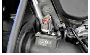
16. Connect the mass air sensor electrical connection.
