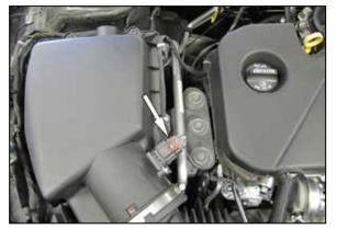
2. Release the red locking tab and then disconnect the mass air sensor electrical connection. Unhook the wiring harness from the air filter housing and set to the side.
