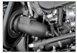
14. Install the K&N<sup>®</sup> intake tube assembly through the heat shield and then into the coupler on the turbo. Adjust the tube and heat shield for best fit and then secure the hose clamp and heat shield bolt.
