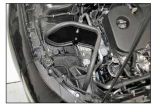
10. Install the heat shield into position and secure with the bolt removed in the previous step.
