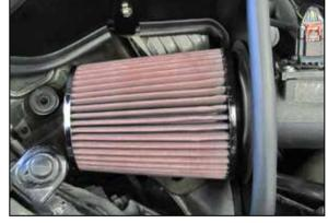
17. Install the K&N<sup>®</sup> air filter and secure with the provided hose clamp.
