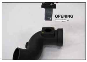
12. Install the mass air sensor assembly into the  $K\&N^{\ensuremath{\circledast}}$  intake tube and secure with the provided hardware.
