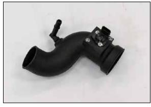
13. Install the provided quick disconnect fitting into the K&N $^{\circ}$  intake tube as shown.
