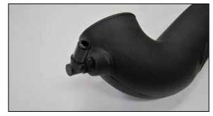
21. Install the 90° quick disconnect vent fitting into the  $K\&N^{\otimes}$  intake tube as shown.
