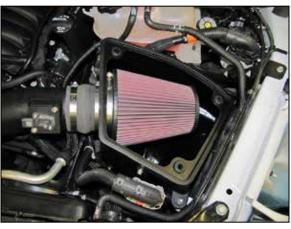
25. Install the K&N<sup>®</sup> air filter onto the filter adapter and secure with the provided hose clamp.
