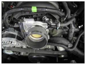
18. On 5.3L vehicles, install coupler #08497 onto the throttle body and secure with the provided hose clamp. On 6.2L vehicles, install coupler #084107 onto the throttle body and secure with the provided
