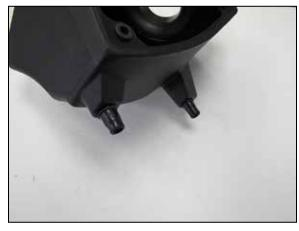
13. Remove the two factory mounting grommets from the factory air filter housing and install them onto the K&N<sup>®</sup> air filter housing.
