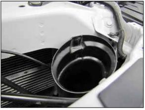
15. Push the factory fresh air intake duct into the  $K\&N^{\circ}$  air filter housing and then reinstall the plastic clip to secure it into position.
