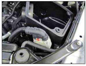
16. Clip the wiring harness onto the bracket installed onto the  $K\&N^{\mbox{\scriptsize \ensuremath{\$}}}$  air filter housing.
