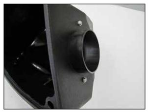
10. Install the provided radius filter adapter into the K&N<sup>®</sup> air filter housing and secure with the provided hardware.
