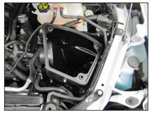
14. Install the K&N<sup>®</sup> air filter housing into the vehicle so the mounting grommets engage into the factory mounting holes. Secure the housing with the factory nut removed in step #9.
