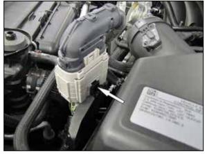
8. Using a small 90° pick or similar tool, release the locking tap that secures the wiring harness bulk connector to the air filter housing and then unhook the connector from the bousing
