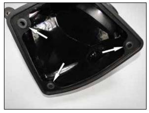
11. Install the three provided grommets into the top of the  $K\&N^{\circ}$  air filter housing.
