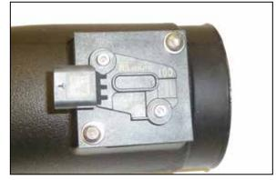
24. Install the mass air sensor assembly into the K&N intake tube and secure with the provided hardware as shown in the photo.
