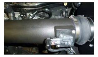
31. Reconnect the mass air sensor electrical connection.
