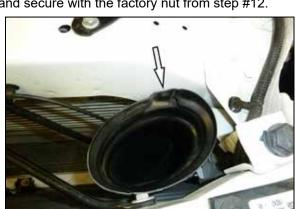
18. Install the fresh air intake duct into the K&N air filter housing and then secure it to the core support using the factory push pin.
