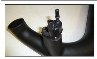
25. Remove the CCV solenoid from the factory intake tube and install it into the K&N intake tube using the factory bolt.
