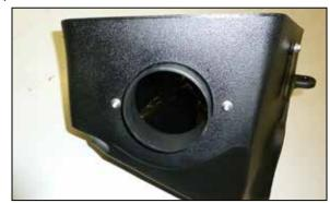
14. Install the filter adapter into the K&N filter housing and secure with the provided hardware.
