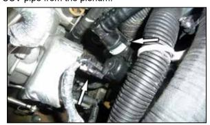
4. Depress the locking tap and then disconnect the CCV pipe from the solenoid attached to the factory intake tube. Disconnect the solenoid electrical connection.
