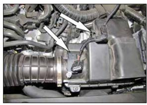
2. Disconnect the Mass air sensor connection and unhook the wiring harness from the air filter housing.
