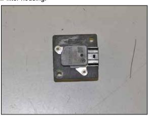
14. Install the mass air sensor into the provided adapter and secure with the provided hardware.
