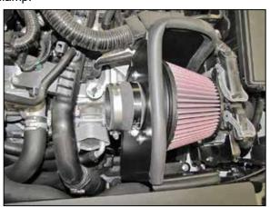
11. Install the coupling hose (084036) onto the filter adapter and secure with the provided hose clamp.
