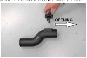
15. Install the mass air sensor assembly into the K&N intake tube and secure with the provided hardware.
