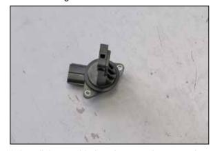
18. Install the provided gasket onto the mass air sensor.
