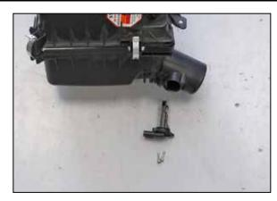
17. Remove the mass air sensor from the factory air filter housing.
