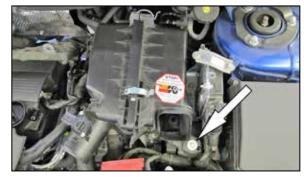
6. Remove the bolt that secures the factory air filter housing to the vehicle. Unhook the brake booster vacuum hose from the air filter housing and then remove the air filter housing from the vehicle. NOTE: K&N Engineering, Inc., recommends that customers do not discard factory air intake.
