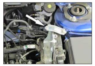
12. Remove the bolt shown that secures the ECU.
