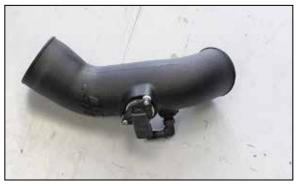
19. Using the four provided washers, install the mass air sensor into the K&N<sup>®</sup> intake tube and secure with the provided hardware.
