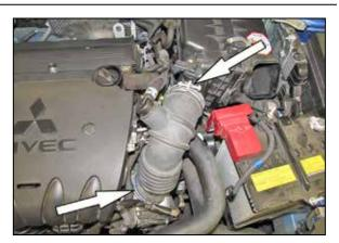
5. Loosen the hose clamps securing the factory intake tube to the air filter housing and throttle body and then remove the intake tube from the vehicle.
