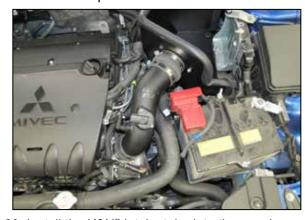
20. Install the K&N® intake tube into the coupler on the filter adapter and then into the coupler on the throttle body. Adjust the tube for best fit and then secure with the provided hose clamps.
