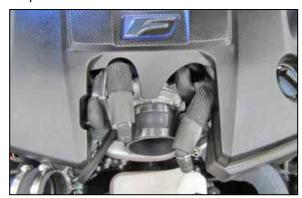
8. Install the coupling hose (084090) onto the throttle body and secure with the provided hose clamp.
