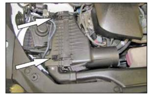
6. Install the  $K\&N^{\otimes}$  air filter and then resecure the clean side housing.
