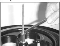
7) Screw the provided all-thread stud into stud adapter until it bottoms out. Secure it with the jam nut.
