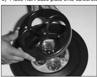
4) Place the K&N Flow Control Stub Stack onto base plate. **NOTE:** make sure the spacer remains in place when placing the stub stack onto the carb post.
