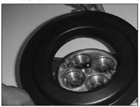
3) Place K&N base plate onto carburetor.
