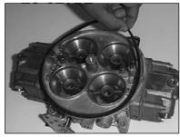
Apply the provided K&N gasket onto carburetor
