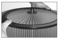
13) Install the X-Steam top making sure it is fully seated on the Filtercharger element all the way around.
