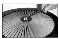
14) Install the provided rubber washer and the flat steel washer. Install the 1/4-20 nylock nut. It should become tight 1-1/2 to 2 turns after contacting the flat washer.
