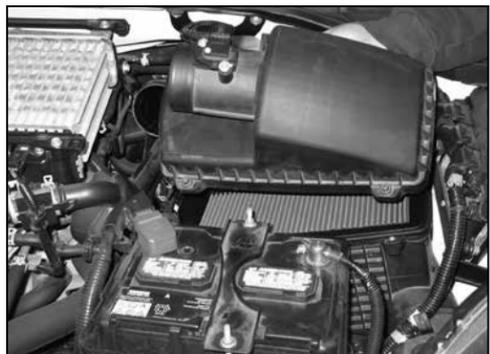
6. Loosen the four bolts that secure the upper airbox housing to the lower airbox housing and then remove the upper airbox housing.
