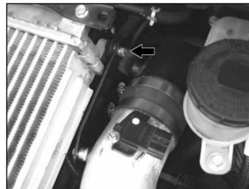
20. Install the K&N® intake tube into the silicone hose at the turbo inlet tube and align so the mounting bracket lines up with the turbo inlet mounting location. Secure the intake tube with the hose clamp and hardware provided.
