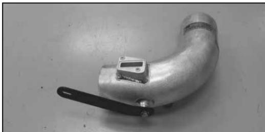
17. Install the supplied tube mounting bracket (070098) onto the K&N® intake tube using the provided hardware.
