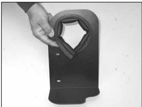
11. Install supplied short edge trim into the hole of the heat shield as shown.
