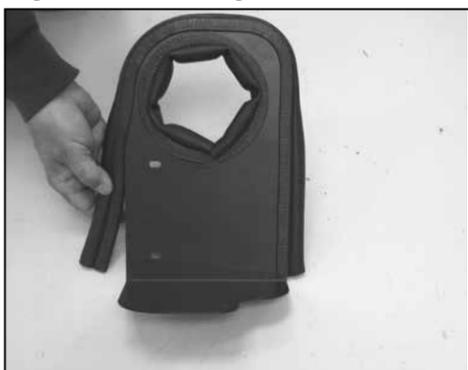
12. Install the long edge trim around the outside of the heat shield as shown.
