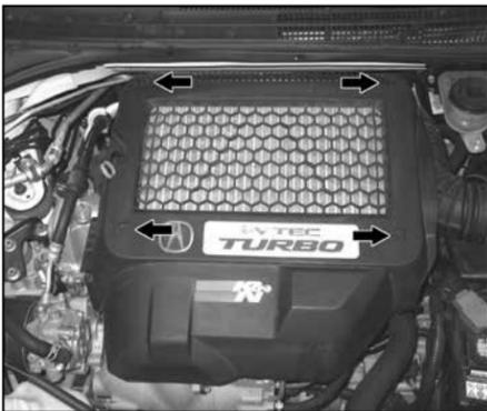
2. Loosen the four quarter turn fasteners that attach the engine cover and lift off the engine cover.
