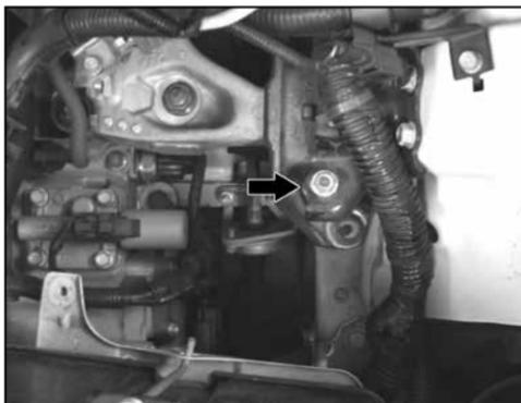
10. Remove the transmission mount bolt shown.
