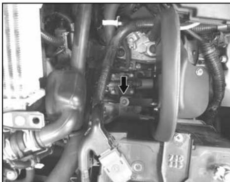
15. Secure the heat shield mounting bracket to the lower airbox mounting tab using the bolt removed in step #7.
