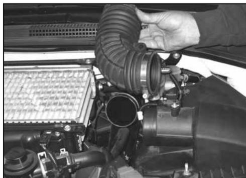
5. Remove the stock intake tube from the vehicle.
