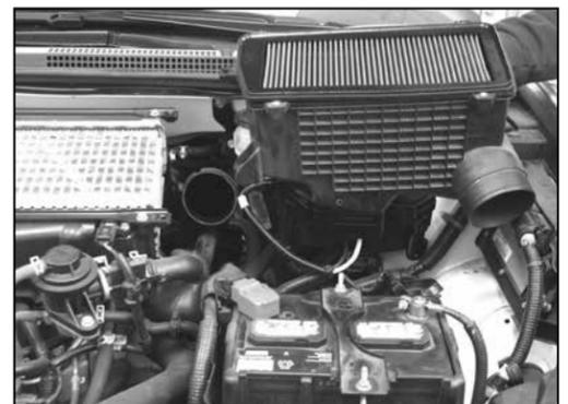
8. Lift and remove the lower airbox assembly.
