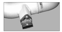
22. Install the MAS into the intake tube using the M5 allen head screws supplied.
