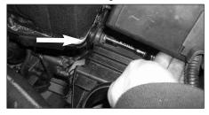
11. Undo the air box mounting nut located on the front of the battery tray as shown.
