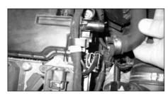
4. Undo the hose clamp and remove the breather hose from the cam cover.
