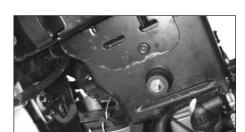
19. Fit the male/male ruber stud to the under side of the fuse and relay box as shown, using a 6mm washer and M6 nylock nut supplied.
