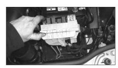
8. Open the fuse and relay box. Unclip the front of the fuse and relay tray and tilt it backwards as shown.
