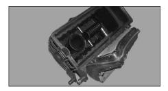
16. From underneath the car, carefully push the air box base upwards from its mounting grommets and remove it from the vehicle.
