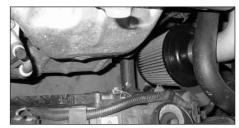
40. This K&N Typhoon intake kit has been designed to be used in two different configurations. In the case of inclement weather, the cold air tube can be removed and the filter can be clamped onto the first intake tube located in the engine compartment as shown to avoid the possibility of ingesting water into the engine.
