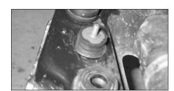
27. Place a large metal washer and the M/F rubber stud over the slot in the lower air box mounting plate as shown.
