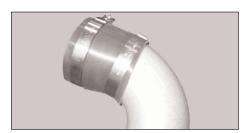
24. Fit the stepped silicone sleeve onto the intake tube using a #40 hose clamp supplied, and fit the #44 hose clamp over the sleeve as shown. Don't fully tighten either yet!
