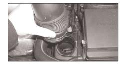
5. Undo the hose clamp and pull the intake tube from the air box as shown.
