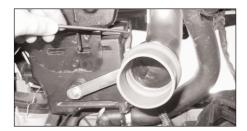
29. Fit the silicone hump hose onto the previously installed intake tube using a #40 hose clamp as shown. Don't fully tighten yet!
