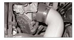
25. Feed the intake tube into the sleeve as shown. Do not fully tighten the #44 hose clamp yet
