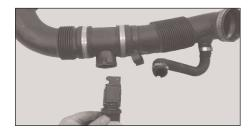
21. Unscrew and remove the MAS from the original intake pipe as shown.
