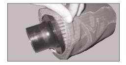
32. Fit the K&N Drycharger over the K&N Filter as shown. **NOTE:** The Drycharger's water repellant properties will last up to 2 years. See parts list to re-order Drycharger if necessary.
