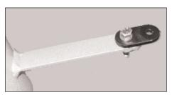
23. Fit the small bracket to the bracket on the intake tube using a M6 bolt, nylock nut and 2 washers supplied. Don't fully tighten yet!
