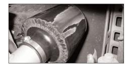
33. Fit the filter onto the "B" tube using the #40 hose clamp supplied as shown. Align filter and "B" tube for best clearance, and fully tighten all the hardware.
