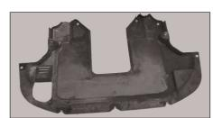
13. Taking all the necessary safety precautions, as per manufacturer's instructions raise the front of the vehicle and support it with axle stands. Then, remove the under tray from the vehicle.
