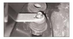
31. Fit the weld-on bracket of the "B" tube onto the rubber stud using a 6mm washer and M6 Nylock nut supplied as shown. Don't fully tighten vet!
