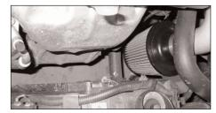
40. This K&N Typhoon intake kit has been designed to be used in two different configurations. In the case of inclement weather, the cold air tube can be removed and the filter can be clamped onto the first intake tube located in the engine compartment as shown to avoid the possibility of ingesting water into the engine.
