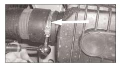
15. From underneath the car, undo the indicated hose clamp as shown and pull the intake snorkel from the air box base.
