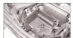
18. Re-install the mounting bracket and fuse and relay box, using their respective original nuts as shown.
