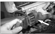
11. **Selespeed models only:** Unclip the indicated cable harness from its bracket as shown.
