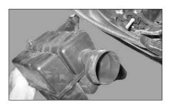
17. Carefully remove the resonator box from the vehicle as shown.
