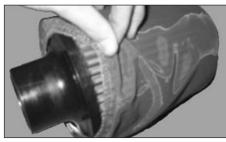
33. Fit the K&N Drycharger over the K&N Filter as shown. **NOTE:** The Drycharger's water repellant properties will last up to 2 years. See parts list to re-order Drycharger if necessary.
