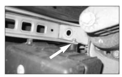
15. From underneath the vehicle, undo and remove the indicated bolt & nut securing the resonator box to the chassis.
