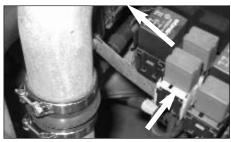
38. With the intake tubes properly aligned and positioned, firmly tighten the hardware securing the mounting bracket.
