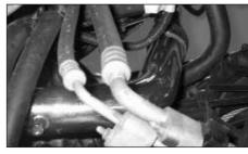
30. From underneath the vehicle, feed the cold air extension tube ( the end without the weld-on stud) into the silicone hump hose as shown but don't tighten the hose clamp yet.
