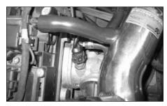
40. Install the breather hose supplied between the vent on the engine and the vent on the intake tube as shown; trim as necessary to eliminate sharp bends in the hose.
