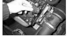
3. Unclip the electrical connector from the Mass Air Sensor (MAS) as shown.
