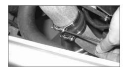
36. Line up the intake tube and cold air extension tube in the silicone hunp hose and fully tighten the hose clamps as shown.
