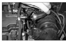
4. Unclip the breather hose from the vent on the engine as shown.
