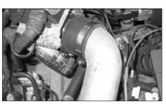
24. Install the intake tube into the silicone stepped hose on the throttle body using a #40 hose clamp supplied as shown. Don't fully tighten yet!
