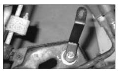
29. Fit the "Z" bracket to the rubber vibration mount as shown, using a Nylock nut and flat metal washer supplied. Don't fully tighten yet!
