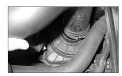
5. Unclip the intake tube and pull it from the air
