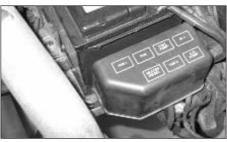
43. Re-install the relay box cover as shown.
