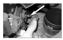
9. Undo and remove the air box securing nut from the threaded stud located under the relay box as shown.
