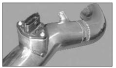
22. Install the MAS into the intake tube using the M5 bolts supplied as shown. **NOTE:** Before installing the MAS, clean the inside of the tube
