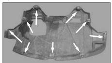
14. From underneath the vehicle carefully remove the under tray from the vehicle.
