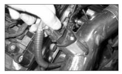
39. Reconnect the electrical connector to the MAS as shown.
