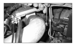
37. Adjust the intake tube for maximum clearance from the battery; now firmly tighten the hosel clamp at the throttle body as shown.
