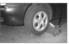
13. As per manufacturer's instructions and taking all necessary safety precautions, carefully raise the front of the vehicle and support it with a pair of axle stands.
