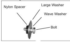
27. Fit first a wave washer, then a large washer and finally the nylon spacer over the shaft of an M6 bolt supplied as shown.
