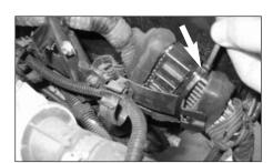
12. **Selespeed models only:** Secure the cable harness between the battery and the bracket using a cable tie supplied as shown.
