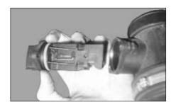
21. Using the provided Torx (69801) unscrew and carefully remove the MAS from its housing as shown
