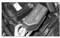
8. Remove the plastic cover from the relay box
