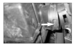
16. Depress the indicated tab to release the resonator box from the air box as shown.
