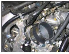
12. Install the provided silicone hose (#08440) onto the throttle body. Secure with the provided hose clamp as shown.
