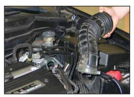
5. Pull firmly to remove the stock intake tube from the airbox. Remove the intake tube from the
