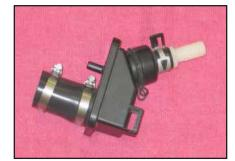
25. Insert the hose mender into the crank case vent chamber. Secure using the stock clamp removed in step # 3.
