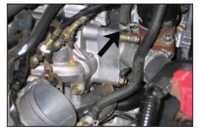
9. Depress the spring clamps on the stock coolant hose at the throttle body and thermostat housing. **NOTE: Ensure the engine is completely cool** before removing the coolant hose, or hot coolant will escape from the cooling system and cause injury or damage.
