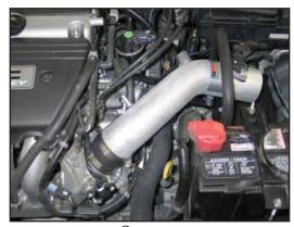
22. Install the K&N<sup>®</sup> intake tube into the silicone hose at the throttle body and align with the tube mounting bracket installed in step # 13. Secure with the provided hardware and hose clamp.
