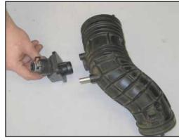
20. Depress the spring clamp and remove the crankcase vent chamber from the stock intake tube.
