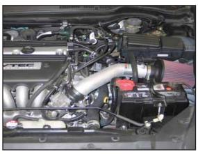
31. Reconnect the vehicle's negative battery cable. Check to ensure all hose clamps and fittings are properly tightened and positioned correctly before starting the vehicle.
