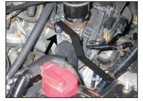
13. Install intake tube bracket (#06498) onto the thermostat housing with the provided hardware as shown.
