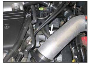
28. Install the stock vent hose onto the  $K\&N^{\ensuremath{\mathbb{R}}}$  intake tube as shown. Secure with the provided hose clamp.
