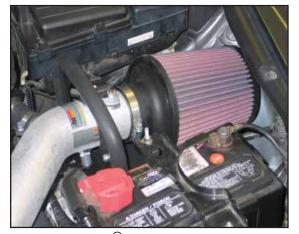
29. Install the K&N<sup>(R)</sup> air filter onto the intake tube as shown.
