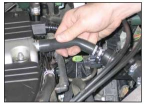
27. Install the crankcase chamber assembly onto the K&N<sup> $\mathbb{R}$ </sup> intake tube and valve cover. Secure with the provided hose clamp.
