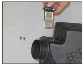
19. Remove the mass air sensor from the stock airbox.
