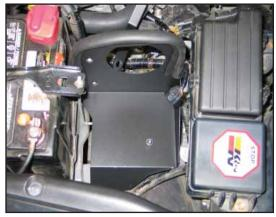
18. Install the heat shield assembly with the provided hardware as shown.
