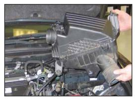
7. Unclip the wiring harness from the bottom of the stock airbox and remove from the vehicle. NOTE: K&N Engineering, Inc., recommends that customers do not discard factory air intake.
