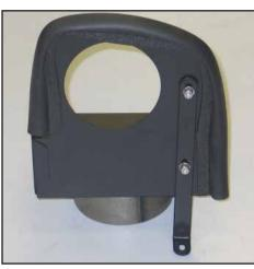
17. Install "L" bracket (#06499) onto the heat shield with the provided hardware as shown.
