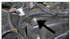
10a. On Acura vehicles, remove the bolt shown that secures the wiring harness mounting bracket to the strut tower.
