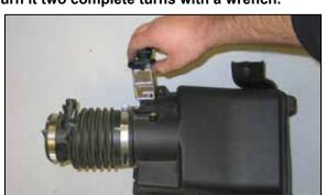
17. Remove the mass air sensor from the stock airbox.
