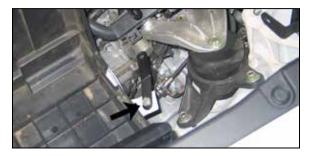
12. Install the heat shield mounting bracket (070115) onto the airbox mounting location on the battery tray using the provided hardware.
