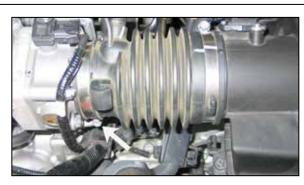
5. Loosen the hose clamp which secures the stock intake tube to the throttle body.
