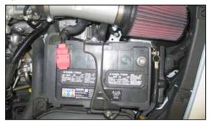
22. Reinstall the battery and secure with the hold down bracket. Reconnect the positive battery cable.
