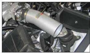
19. Install the K&N® intake tube into the silicone hose at the throttle body and align with the mounting bracket. Secure with the hose clamp and provided hardware.
