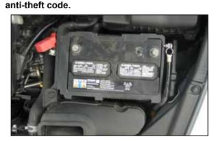
2. Disconnect the positive battery cable, remove the battery hold down and then remove the battery.
