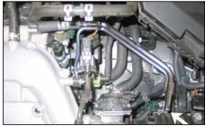
4. Disconnect the crankcase vent tube from the intake tube and valve cover port as shown. The spring clamps will not be reused.
