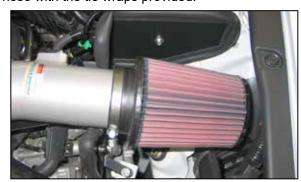
21. Install the K&N® air filter onto the intake tube and secure with the provided hose clamp.
