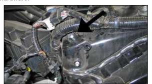
11a. On Acura vehicles Install the heat shield mounting bracket (083158) onto the strut tower and secure with the provided hardware.
