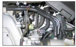
20. Install the provided crankcase vent hose onto the NPT fitting and then onto the valve cover port. Secure the crankcase hard line to the provided hose with the tie wraps provided.
