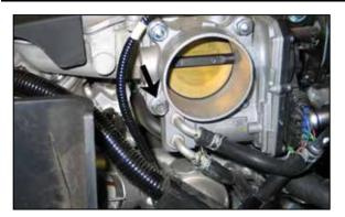
8. Remove the front lower throttle body bolt shown. **NOTE: This bolt will be reused in the next step.**
