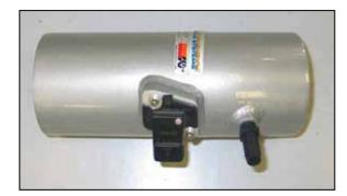
18. Install the mass air sensor into the K&N<sup>®</sup> intake tube and secure with the provided hardware.
