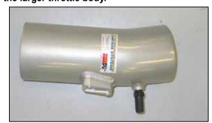
16. Install the  $\frac{1}{4}$ " NPT fitting into the K&N® intake tube as shown.
