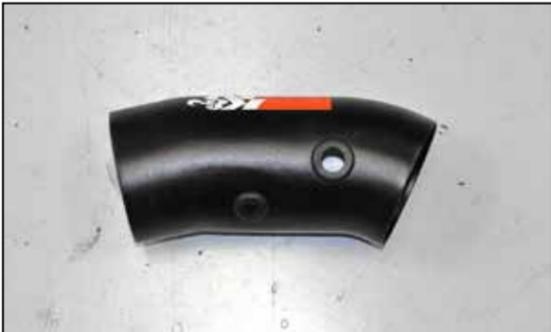
11. Install the two provided grommets into the K&N® intake tube.
