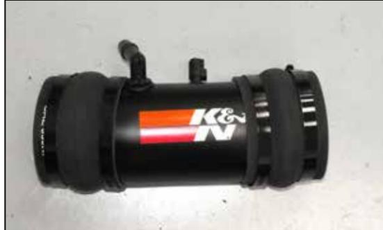
14. Install both coupling hoses (08418) onto the K&N® intake tube as shown.
