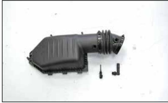
12. Remove the crank case vent and inlet air temperature sensor from the factory intake tube.
