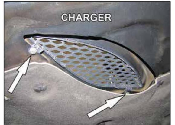
18. If the vehicle is to be driven during inclement weather it is recommended the shield be installed onto the hood vent to guard, the air filter from concentrated water. Remove the two bolts that secure the factory vent grid.
