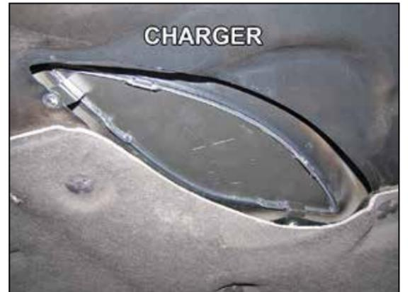
19. Install the guard so the mounting tabs are between the hood and the factory grid as shown.
