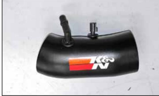
13. Install the crank case vent and inlet air temperature sensor into the K&N® intake tube.
