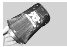
24. Fit the Drycharger around the filter. **NOTE:** The Drycharger's water repellant properties will last up to two years. See the parts list to re-order Drycharger if necessary.
