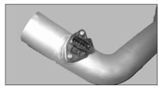
14. Install the MAS into the the K&N Typhoon A-tube using the two M5 screws supplied. **NOTE:** Before installing the MAS, inspect the inside of the tube for any debris or dirt and clean as necessary!
