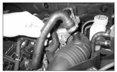
3. Remove the breather hose from the engine and the intake tube.
