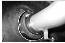
25. Fit the filter/drycharger assembly through the hole in the, onto the B-tube using the #48 hose clamp supplied. Ensure that the filter has sufficient clearance in the hole. If not, enlarge the hole as necessary.
