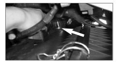
9. From underneath the vehicle, unscrew the air box mounting bolt from the mounting underneath the battery tray.
