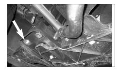
13. Remove the rubber grommet on the left side and mount the rubber vibration stud using the two large washers and the M6 nylock nut supplied. Make sure to fit a large washer either side of the hole & do not fully tighten yet!
