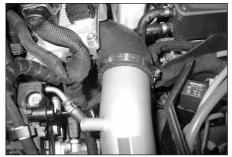
16. Slide the A -tube into the silicone hose using a #325 barrel clamp supplied. Do not fully tighten yet!
