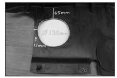
22. Cut a hole into the left under tray (removed in step 8)with a diameter of approx. 135mm at 65mm from the top and 15mm from the side as shown.
