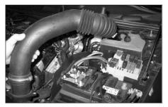
5. Unscrew and remove the complete intake tube including the MAS from the throttle body as shown.
