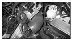
15. Mount the 90 degree silicone hose onto the throttle body using a #325 barrel clamp supplied. Do not fully tighten yet!
