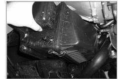
10. Carefully push the airbox upwards, out of its mounting grommets, and carefully remove it from the vehicle as shown.
