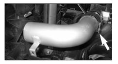
20. Fit the B-tube into the silicone hump hose using a #300 barrel clamp supplied. Do not fully tighten yet!
