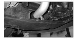
23. Re-install the left under tray to the vehicle as shown using its original hardware.
