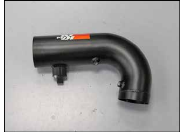
19. Install the mass air sensor into the K&N® intake tube and secure with the provided hardware.
