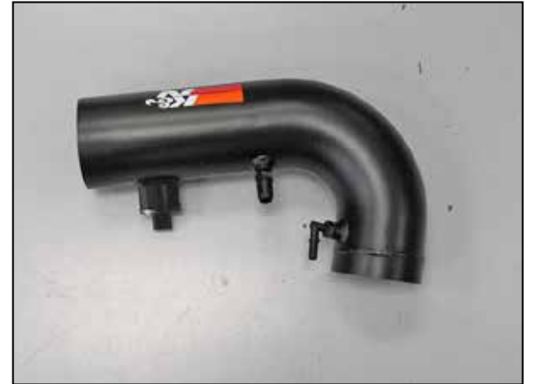
20. Install the two vent fittings into the K&N® intake tube as shown.
