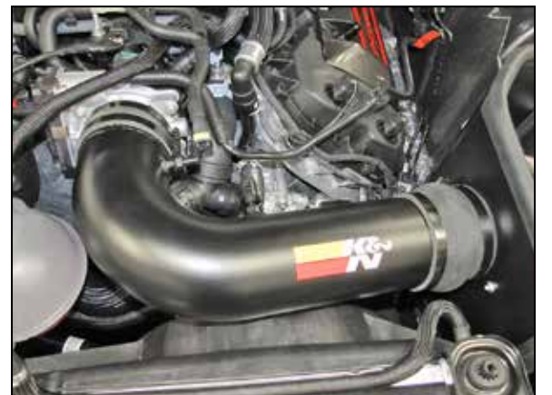
21. Install the K&N® intake tube into the coupler at the filter adapter and then into the coupler at the throttle body, adjust the tube for best fit and then secure with the provided hose clamps.
