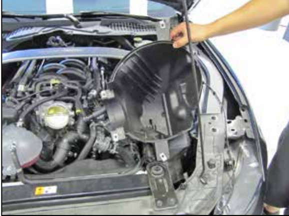
8. Remove the lower heat shield from the vehicle. NOTE: K&N Engineering, Inc., recommends that customers do not discard factory air intake.
