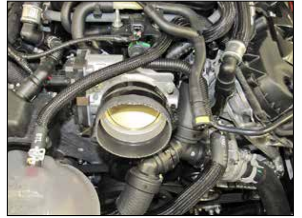
17. Install the provided coupler (08618) onto the throttle body and secure with the provided hose clamp.
