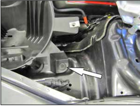
7. Remove the bolt shown that secures the lower heat shield to the inner fender.
