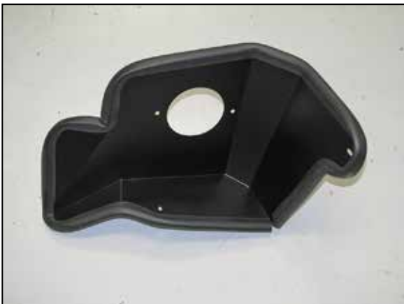
11. Install the provided edge trim onto the heat shield as shown. NOTE: Some trimming of the edge trim will be necessary.
