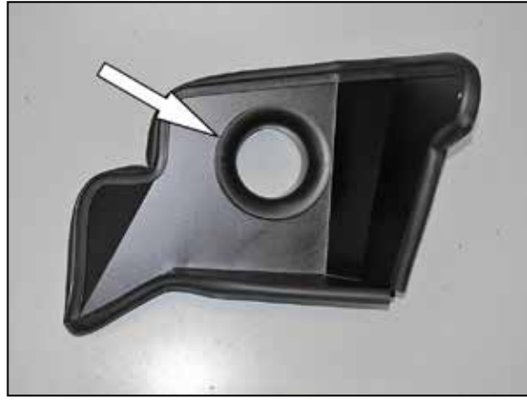
12. Install the filter adapter into the heat shield and secure with the provided hardware.
