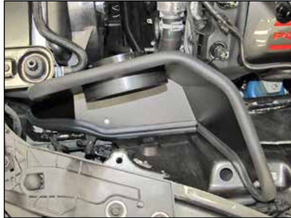
14. Install the heat shield onto the lower mounting bracket and secure it to the mounting bracket only with the provided hardware.
