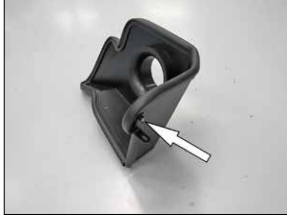
13. Install the provided heat shield bracket (064326) onto the heat shield and secure with the provided hardware.
