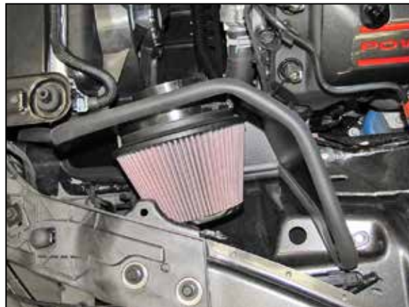
15. Lean the heat shield in enough to install the K&N® air filter onto the adapter and secure the filter with the provided hose clamp. Then secure the heat shield mounting bracket to the inner fender with the provided hardware.
