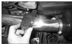
14. Reconnect the mass air sensor electrical connection as shown.
