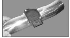
9. Install the mass air sensor into the K&N Typhoon intake tube using the stock bolts from step 8. NOTE: Before installing the mass air sensor, inspect the inside of the tube for any debris, then clean the inside out with water and a towel. Inspect the tube one more time before proceeding to the next step
