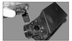
8. Remove the two bolts that secure the mass air sensor, then, remove the mass air sensor as shown.
