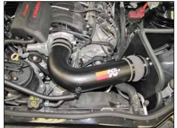
19. Install the intake tube into the Hump hose and then into the hose at the throttle body, adjust the tube for best fit and then secure with the provided hose clamps.
