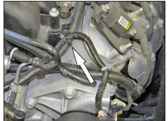
21. Connect the mass air sensor electrical connection and then secure the wiring harness to the engine harness with the provided tie wrap.
