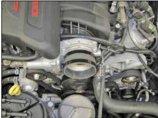
14. Install the provided coupler hose #08761 onto the throttle body and secure with the provided hose clamp.
