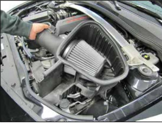
7. Lift up the air filter housing to dislodge it from the inner fender and then remove it from the vehicle.
