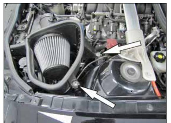
6. Remove the two nuts securing the air filter housing to the inner fender.
