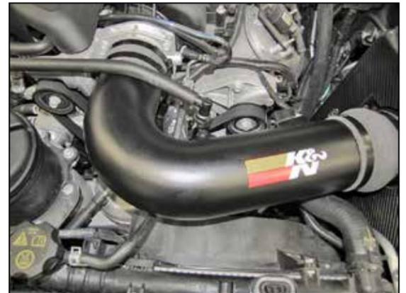
20. Connect the stock ccv hose the quick disconnect fitting installed into the intake tube.
