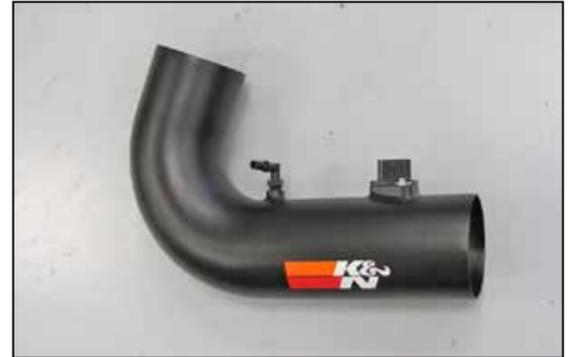
18. Install the 90° NPT quick disconnect npt fitting into the K&N® intake tube as shown.
