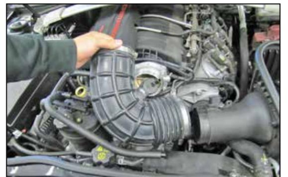
5. Loosen the hose clamps securing the intake tube to the throttle body and mass air sensor then remove the intake tube from the vehicle.
