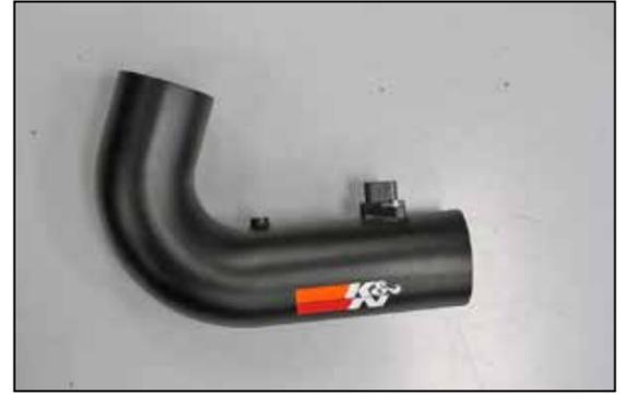
17. Install the mass air sensor into the K&N® intake tube and secure with the provided hardware.
