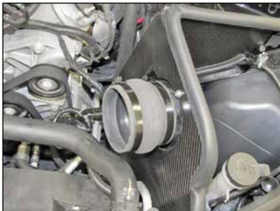
15. Install the provided hump coupler hose #08418 onto the filter adapter and secure with the provided hose clamp.
