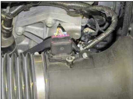
2. Disconnect the mass air sensor electrical connection and unhook the wiring harness from the intake tube.
