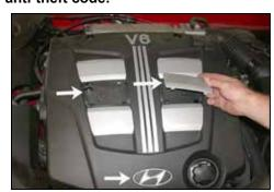
2. Remove the three engine cover panels using a flat blade screwdriver.
