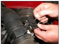
5. Remove the wire clip, then, disconnect the mass air sensor electrical connection as shown.
