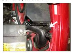
14. Remove the bolt that secures the air cleaner duct to the inner fender as shown.
