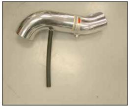
20. Install the provided hose onto the K&N $^{\! \otimes}$  intake tube as shown.
