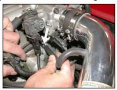
22. Connect the crank case vent hose to the crank case vent as shown.
