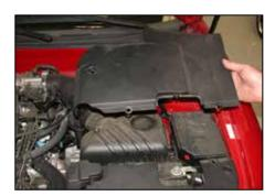
4. Remove the two plastic rivets and one bolt, then, remove the air cleaner cover as shown.
