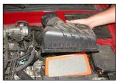
8. Unclip the air cleaner cover and remove as shown.
