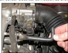
6. Disconnect the crank case vent hose and remove from the engine as shown.
