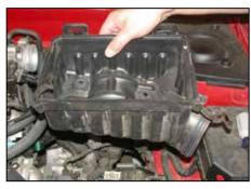
9. Remove the lower air cleaner assembly, which is secured by three bolts.
