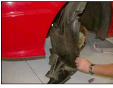
12. Remove five plastic rivets and one bolt, then, pull in the inner fender valance down as shown.
