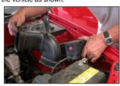
16. Remove the fuse box bolts, lift upward, then, remove the air cleaner duct as shown.
