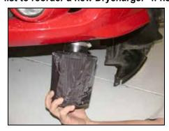
30. Install the K&N $^{\circ}$  air filter from under the vehicle and secure with the provided hose clamp as shown
