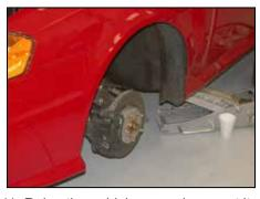
11. Raise the vehicle up and support it with a jack stand, then, remove the front tire as shown.
