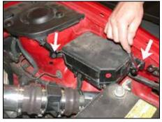
31. Secure the fuse box using the original bolts.
