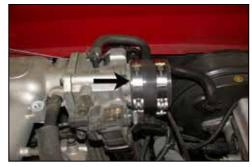
17. Install the silicone hose and hose clamps onto the throttle body and secure as shown.
