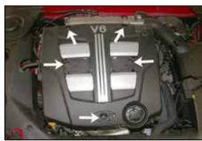
3. Remove the engine cover, which is secured by 5 bolts as shown
