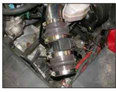
25. Slide the mass air sensor assembly onto the throttle body tube and snug the hose clamp but do not tighten completely at this time.
