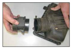
23. Remove the mass air sensor from the air cleaner cover as shown.
