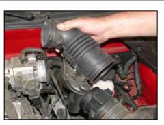
7. Loosen the hose clamps at the throttle body and at the mass air sensor, then, remove the stock intake tube as shown.
