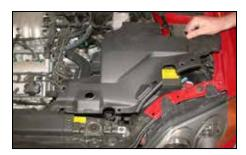
10. Remove the battery cover, which is secured by 4 plastic rivets and one bolt as shown.
