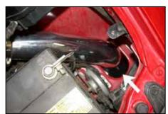
27. Slide the cold air tube through the fender from underneath the vehicle and into the silicone hump hose as shown.
