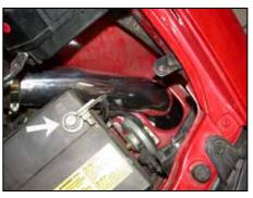
35. Reconnect the negative battery cable and double check that everything is tight and properly positioned before starting the vehicle.
