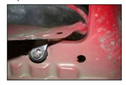
28. Line up the cold air tube bracket with the rubber mounted stud from step 26 and secure with the provided hardware as shown.
