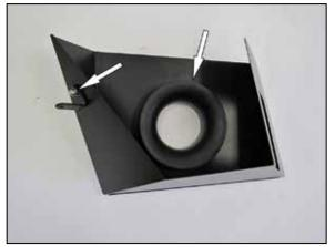
9. Install the provided heat shield mounting bracket and filter adapter onto the heat shield and secure with the provided hardware.
