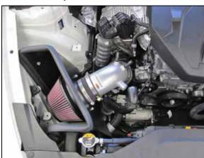
14. Install the heat shield assembly and intake tube as a unit into the vehicle. Secure the heat shield using the provided hardware. Adjust the intake tube for best fit and secure with the provided hose clamps.
