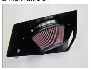
10. Install the air filter onto the heat shield and secure with the provided hose clamp.
