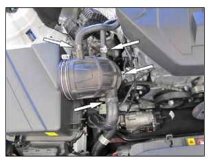
3. Disconnect the vent lines attached to the factory intake tube. Loosen the hose clamp that secures the intake tube to the turbo inlet and then remove the upper housing and intake tube from the vehicle.
