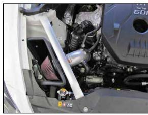
16. Reinstall the chassis brace and secure with the factory hardware.
