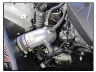
15. Connect the vent lines to the K&N® intake tube as shown.
