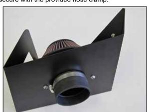
11. Install the provided coupler (08698) onto the filter adapter and secure with the provided hose clamp.
