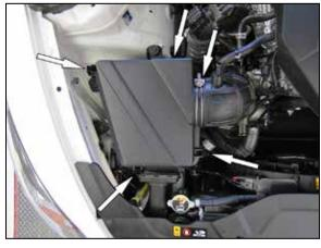
4. Release the four-upper air filter housing retaining clips and loosen the hose clamp that secures the housing to the intake tube. Remove the upper housing from the vehicle.
