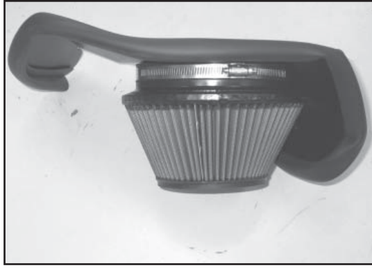
28. Install heat shield onto filter assembly as shown.
