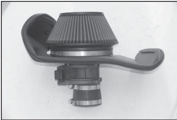
30. Attach the silicone hose to the MAF sensor with the provided hose clamps. NOTE: The hose clamp ratchets are on the same side as the MAF hookup.
