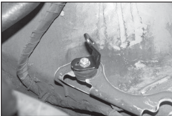
32. Install assembled bracket on lower air box mount. NOTE: The two large washers should sandwich the smaller hole to hold the bracket in place.
