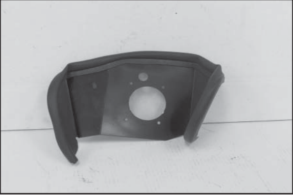
24. Install the provided edge trim to the heat shield.
