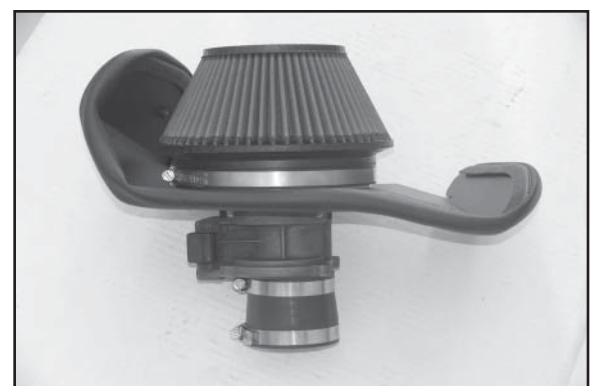
22. On the factory air intake tube, loosen the clamp to remove the MAF to the factory air intake tube.
