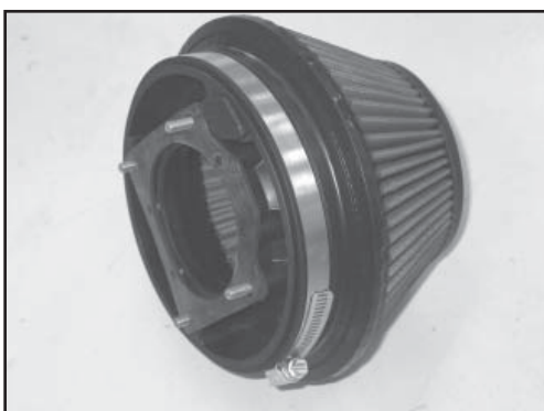
27. Install adaptor to filter and secure as shown.
