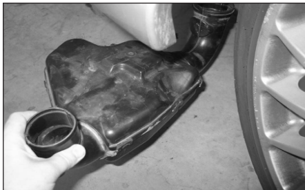
10. Remove the resonator box from the vehicle as shown by pulling it backwards.
