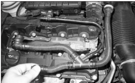
3. Remove the breather assembly from the vehicle as shown; press the yellow tabs to release.
