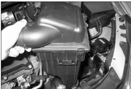
5. Remove the complete air box assembly from the vehicle by pulling it firmly upwards.
