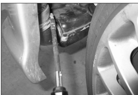
9. Unclip the indicated hose clamp securing the intake snorkel to the resonator box.
