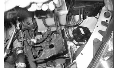
13. Remove the complete airbox mounting bracket by pulling it upwards.
