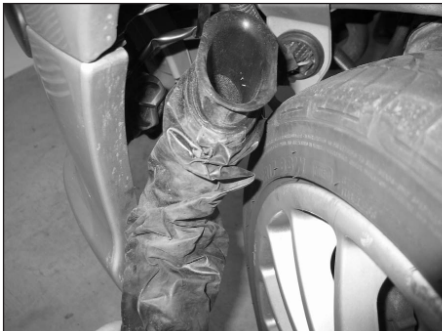
11. Carefully remove the cold air intake snorkel from the inner wing as shown.
