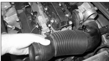
4. Unclip and remove the intake hose from between the throttle body and air box.
