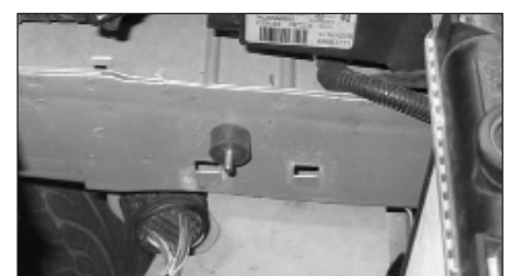
14. Screw the rubber vibration stud provided into the threaded air box mounting point from step 12 as shown.
