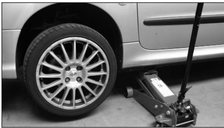
7. Taking the necessary safety precautions raise the front of the vehicle as shown and support the vehicle with axle stands.
