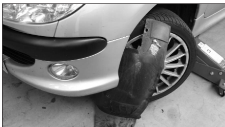
8. Remove the wheel arch liner from the vehicle as shown by removing the clips and 2 Torx screws using the small wrench provided.
