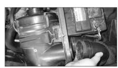
5. Disconnect the 2 air box feed pipes from the air box as shown.
