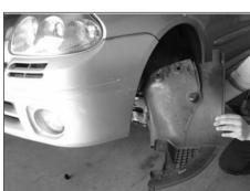
24. Re-install the wheel arch liner using its original hardware. Now re-install wheel to the vehicle. Re-install the front wheel and torque it up to factory specifications!
