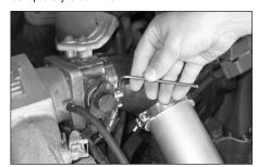
18. Fit the silicone hose on to the throttle housing using the #325 barrel clamp supplied. Don't fully tighten yet!
