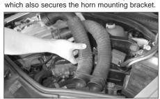
13. Remove the air box intake pipes from the vehicle. Re-install the horn mounting bracket removed in the previous step using its original
