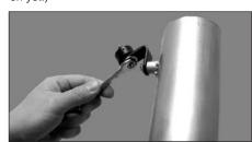
15. Fit the vibration mount on to the bracket using an M6 nylock nut & washer supplied.
