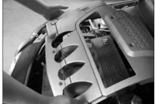
2. Unbolt and remove the engine cover from the vehicle
