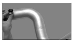
14. Fit the bracket onto the threaded standoff on the new intake pipe using the M6 bolt and M6 waved washer supplied. (do not fully tight-
