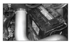
22. Re-install the battery to the vehicle and reconnect the battery terminals (positive terminal first).
