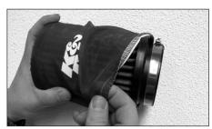
19. Fit the drycharger on to the filtercharger as shown. **NOTE:** The Drycharger's water repellant properties will last up to two years. See the parts list to order Drycharger if necessary.
