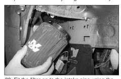
20. Fit the filter on to the intake pipe using the #44 hose clamp supplied. Align the complete intake tube assembly for maximum clearance. Now firmly tighten all hose clamps and hardware.
