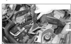
9. Unbolt & remove the air box support bracket and re-install the rear bolt.
