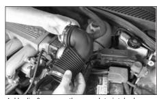
4. Unclip & remove the complete intake hose assembly.
