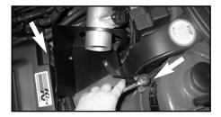
18.Mount the heat shield onto the air box support points using the hardware supplied. ( do not fully tighten yet!)
