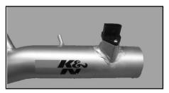
14. Mount the MAS onto the new intake tube using the two M5 bolts supplied. **NOTE**: Before installing , inspect the inside of the tube for any debris, then clean the inside out with water and a towel.
