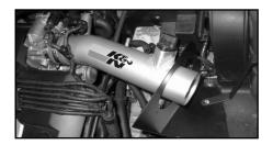
19. Align the tube and the bracket for best clearance. Now remove the heat shield assembly, keeping the tube and bracket in place.
