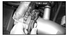
25. Zip tie the crank case vent switch connection to the trottle control connection using the provided cable tie as shown.
