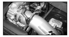
16. Fit the new intake tube into the silicone hose using the #325 barrel clamp supplied. (do not fully tighten at this moment.)
