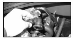
6. Disconnect the crank case vent switch and the crank case hose from the intake tube as shown.
