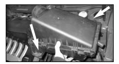
4. Remove the two bolts securing the air box and remove the complete airbox.
