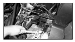
9. Remove the gear mounting bolt as shown.
