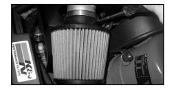
26. Fit the filter onto the intake tube using the hose clamp supplied.
