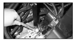
20. Now firmly tighten the gear box mounting bolt and the M6 bolt on the intake tube.
