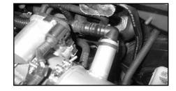
23. Reconnect the crank case vent hose to the intake tube.
