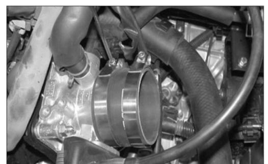
28. Install the silicone hose and hose clamps onto the throttle body and secure as shown.
