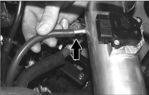
32. Connect the EVAP OBD canister closed valve to the vent on the K&N® Typhoon® intake tube as shown.
