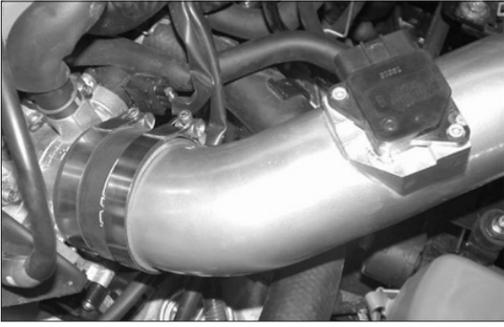
29. Slide the K&N® Typhoon intake tube into the silicone hose on the throttle body as shown. Do not tighten completely at this time.
