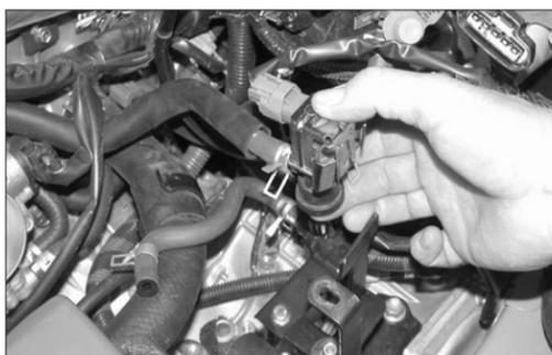
22. Disconnect the vent hose on the PWM vacuum switching valve, then, reroute the hose in front of the cruise control cable and reconnect as shown.
