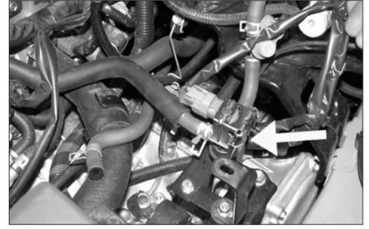
23. Slide the PWM vacuum switching valve onto the T-bracket as shown.
