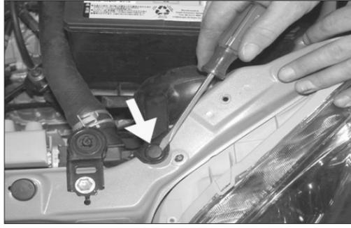
16. Remove the push clip that secures the air inlet duct to the radiator core support as shown.
