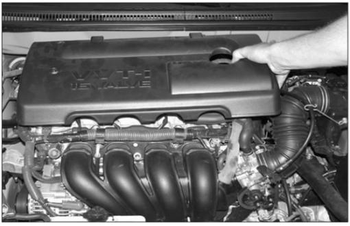
3. Remove the engine cover as shown.
