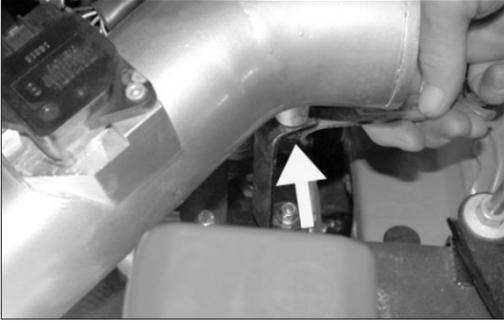
30. Line up the K&N® Typhoon® intake tube with the "C" bracket and adjust the bracket for best fit, then, secure the tube to the bracket with the provided hardware.
