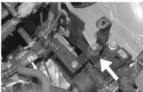
21. Secure the provided "C" bracket to the rubber mounted stud using the provided hardware. Do not tighten as some adjustment will be necessary.
