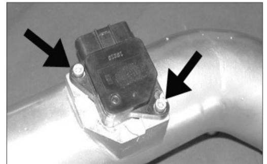
27. Install the mass air sensor into the K&N® Typhoon® intake tube using the provided hardware as shown.
