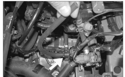
25. Install the provided silicone hose onto the EVAP OBD canister closed valve as shown.
