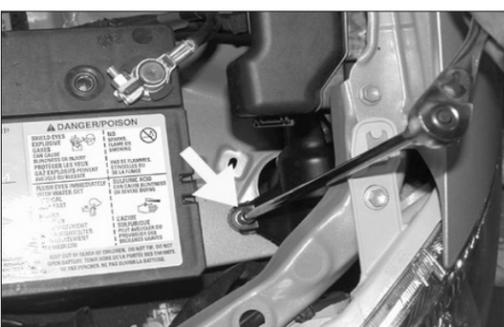
15. Remove the bolt that secures the air inlet duct to the inner fender as shown.
