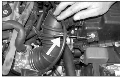
5. Remove the throttle cable from the stock wire hanger as shown.
