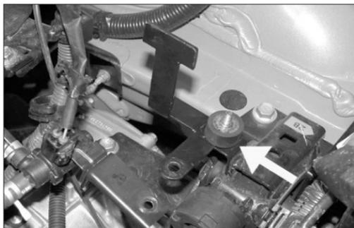
19. Secure the provided T-bracket to the stock air cleaner mount using the provided rubber mounted stud.
