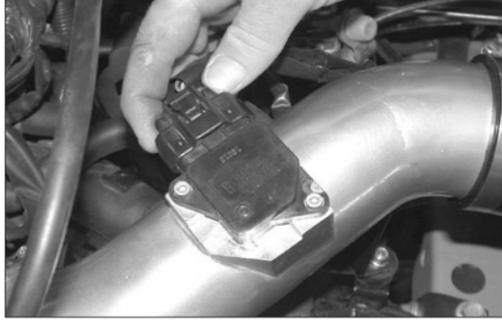
34. Reconnect the mass air sensor electrical connection as shown.
