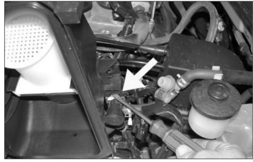
8. Unclip the upper air cleaner assembly and tilt it upward, then, using a flat blade screwdriver depress the release tab on the air cleaner assembly to release the PWM vacuum switching valve as shown.
