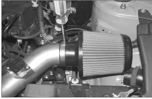
33. Install the K&N X-Stream air filter onto the K&N® Typhoon intake tube as shown.
