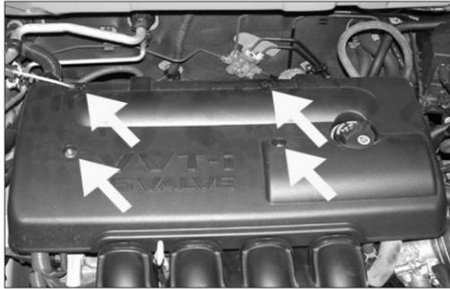
35. Reinstall the stock engine cover using the stock acorn nuts and the provided button head screws to replace the stock push clips.
