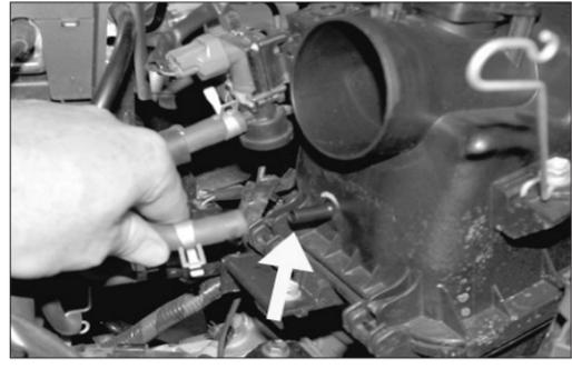
7. Disconnect the EVAP OBD canister closed valve vent hose from the air cleaner assembly as shown.
