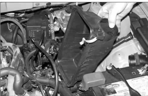
13. Remove the lower air cleaner assembly as shown.
