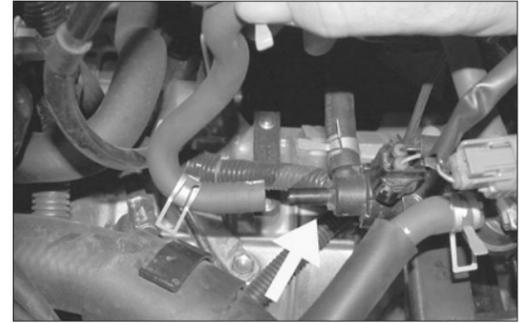
24. Remove the vent hose from the EVAP OBD canister closed valve as shown.
