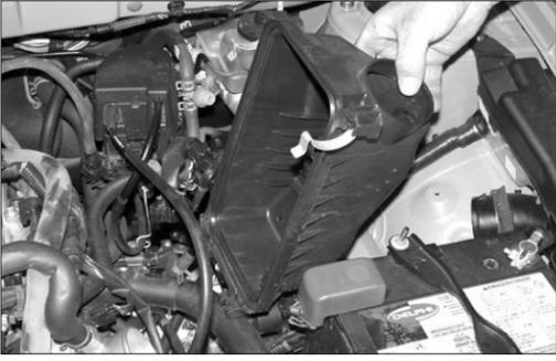
10. Remove the three bolts that secure the air cleaner assembly, then tilt the air cleaner assembly upward as shown.
