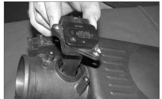
26. Remove the mass air sensor from the upper air cleaner assembly as shown.
